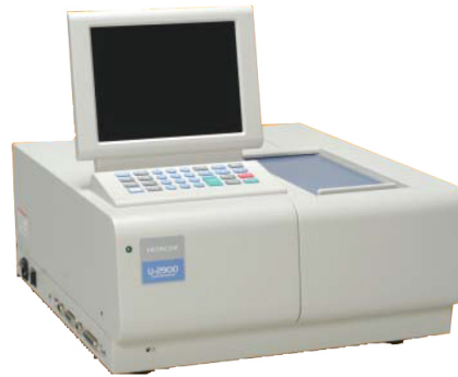
Figure 2.2: Double beam UV spectrophotometer used to measure the absorption spectrum of aqueous KCl solution.
