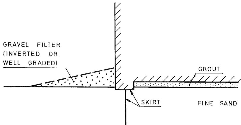
Figure 3.2: Use of filter to reduce exit gradient.
