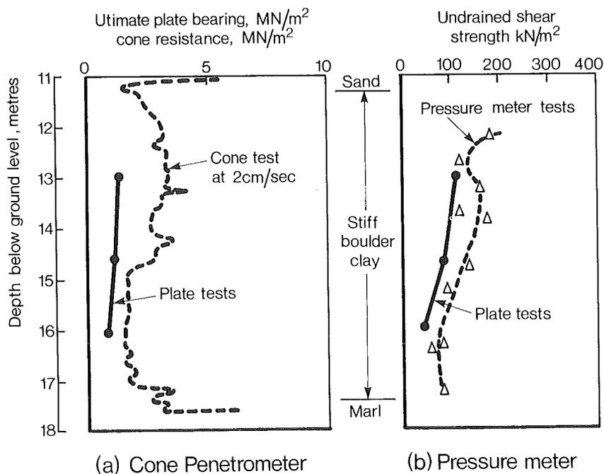
Figure 2.6: Comparison of soil strength from different in situ tests.
