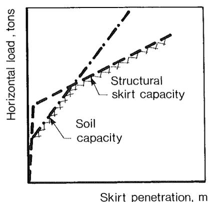
Figure 4.4: Soil and skirt capacity at different penetration depths.
