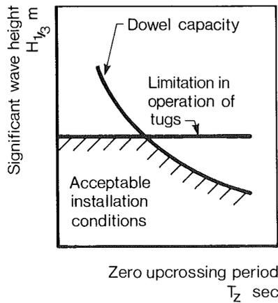
Figure 4.1: Sea state conditions for installation.
