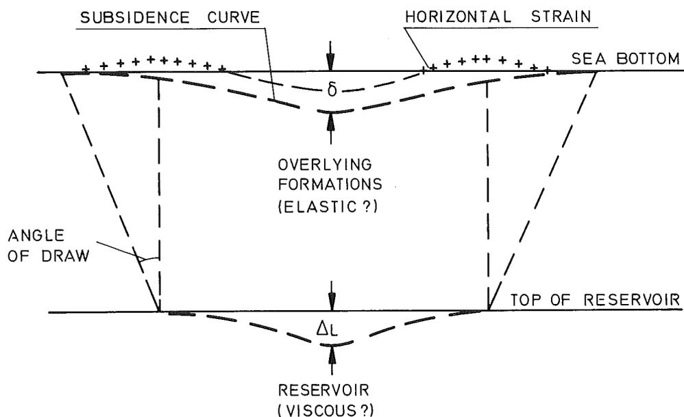
Figure 3.4: Sketch of subsidence due to assumed drop in fluid (or gas) pressure in the producing reservoir.
