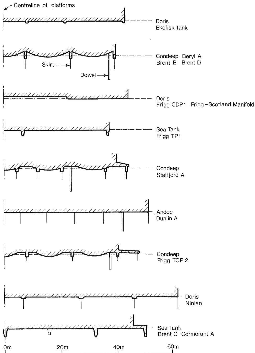
Figure 4.5: Bottom sections of concrete platforms in the North Sea.
