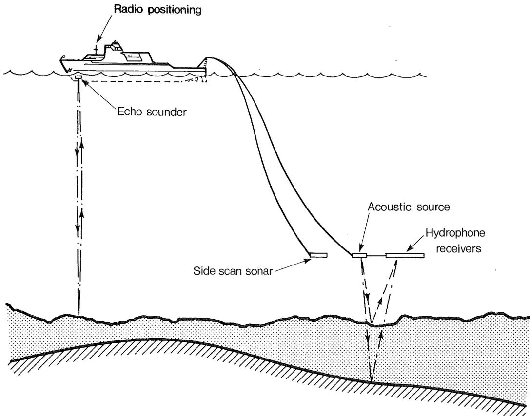
Figure 2.2: Diagram of towed seismic devices.
