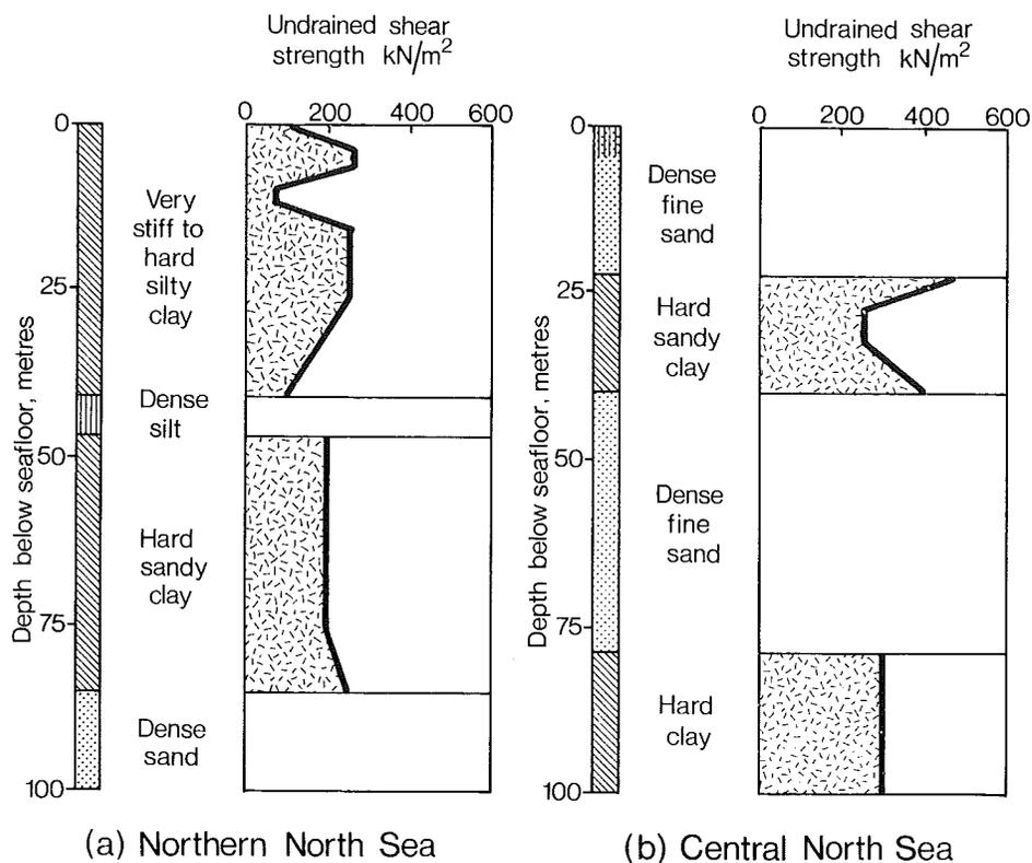
Figure 2.1: Typical soil profiles.
