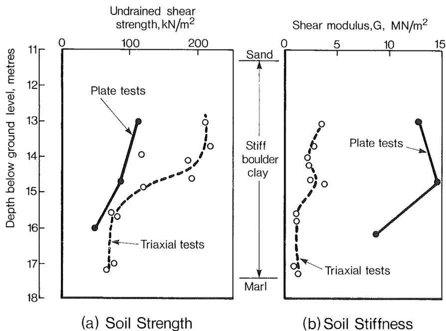
Figure 2.7: Comparison of results from deep plate load tests and laboratory tests.
