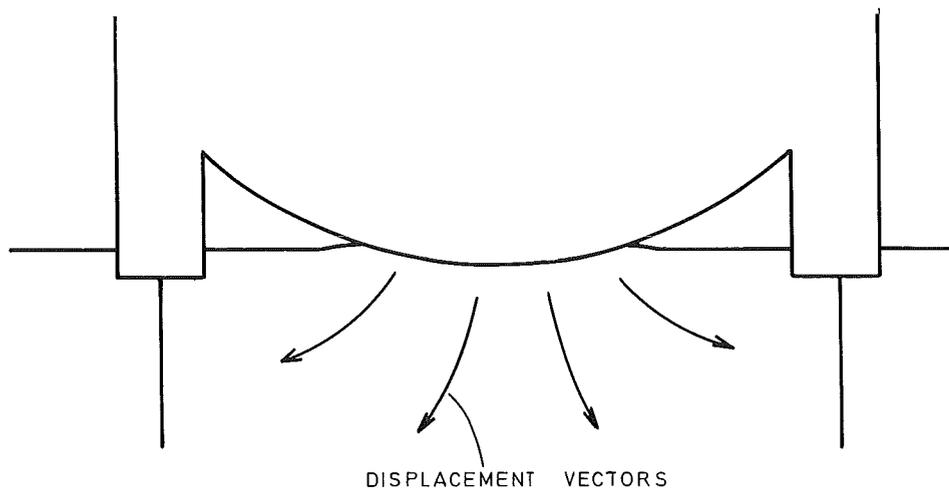
Figure 3.8: Lateral loads on skirts due to dome penetration.
