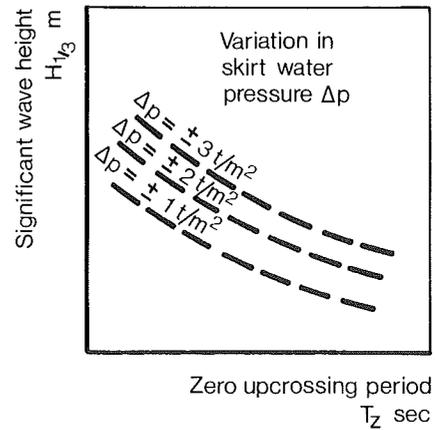
Figure 4.2: Variation in skirt water pressure caused by over-turning moment from sea state.
