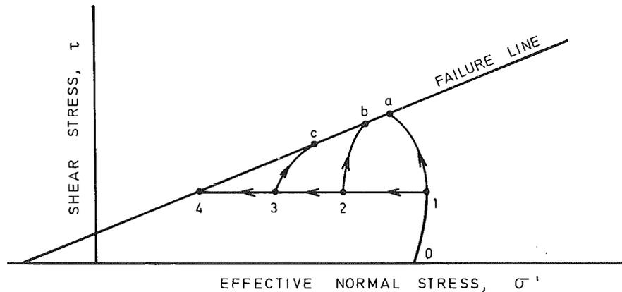
Figure 3.9: Effects of repeated loading on soil behaviour.
