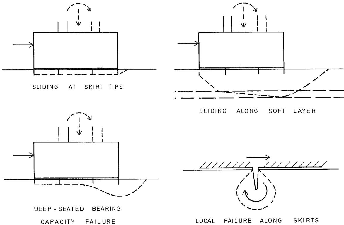
Figure 3.1: Examples of failure modes.
