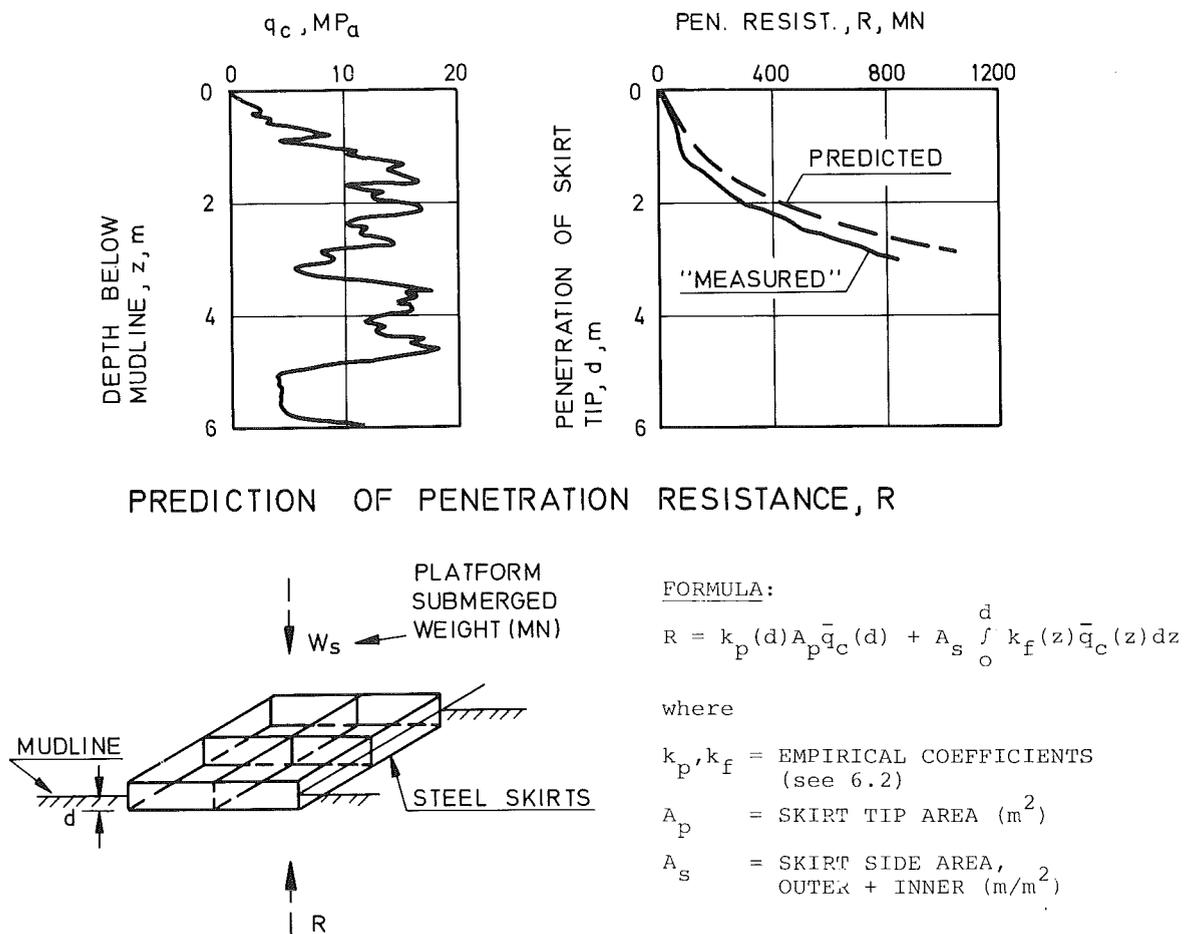
Figure 3.7: Approach for prediction of penetration resistance of steel skirts and dowels.
