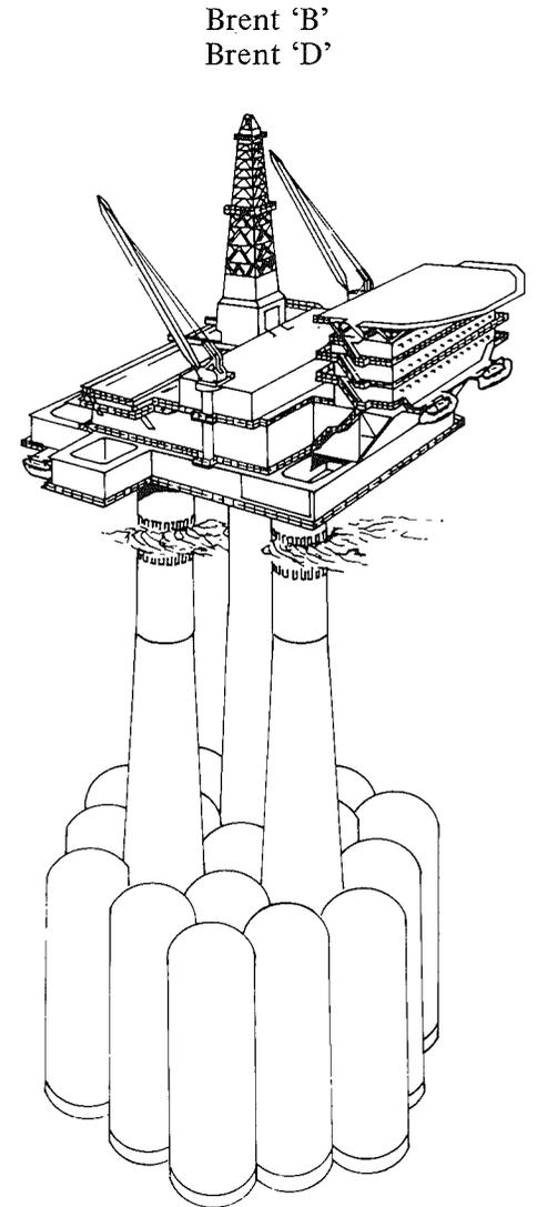
Figure 1.4: Concrete platforms used by Shell Expro.
