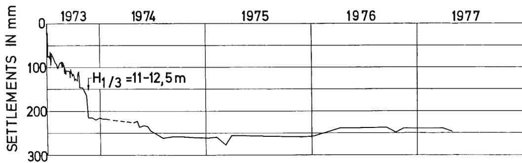
Figure 3.5: Observed settlements of the Ekofisk tank.
