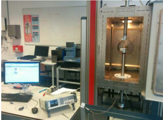
Figure 15: This figure shows the experimental set-up of both experiments, although the LCR is not used during repeatability testing. The PC is used to control the UTM (on the right). The heat chamber is the compartment surrounding the clamps of the UTM. For the self-sensing experiment the LCR is used, is connected to the PC on one end and to the TCPM via the clamps on the other end.
