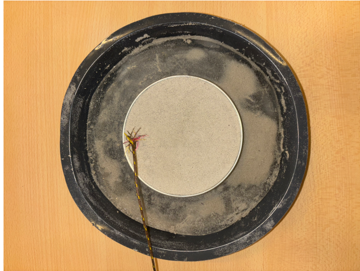
Figure 4.1: Set-up of the frozen quartz sand sample with a layer of ice around the container. The sample has a hole in which the thermal couple is placed.
