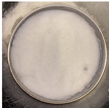
(b) Ice analogue that has spent 190h in -25^{\circ}\text{C} freezer.
