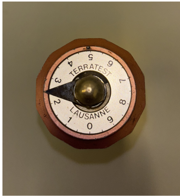
Figure 4.3: Top view of the pocket shear vane test instrument indicating the shear strength values.
