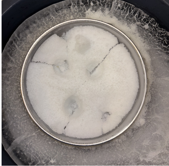
(a) The -25 °C analogue after strength testing with t_f = 190 hours.
