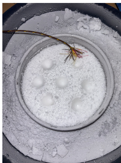
(b) An example of what the measurements look like on an ice analogue using the CONE method. This is a -80^{\circ}\text{C} analogue with 7 measurements.
