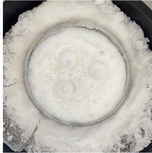
(b) The -80 °C analogue after strength testing with t_f = 190 hours.
