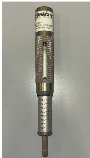
Figure 4.4: Pocket penetrometer tool used to measure the compressive strength of a soil.
