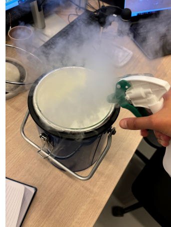
Figure 3.2: Close-up of the process of spraying water into the dewar
