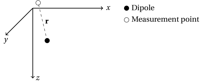
Figure 8.1: Illustration of a single dipole and a single measurement point. The dashed line shows the vector \mathbf{r} that connects the dipole and the measurement point.
