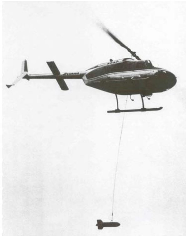
Figure 7.1: A bird installation on a helicopter. The magnetometer is attached to a rope, which is attached to the helicopter. The magnetometer is therefore less sensitive to the platform field of the helicopter. This figure is taken from [54].
