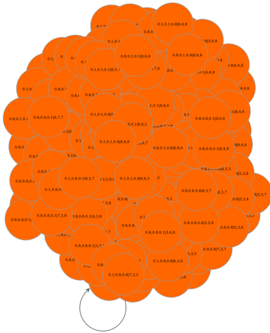
Figure C-1: The l -complete abstraction S_{Q/Q_3} of depth l = 3 visualized as Transition System (TS), using two monotone Lyapunov triggering conditions with decay rates: 0.1, 0.8 and a maximum discrete IST of k_{max} = 8 . In the quotient states, one can see the trigger condition sequence on the left and the IST sequence on the right.
