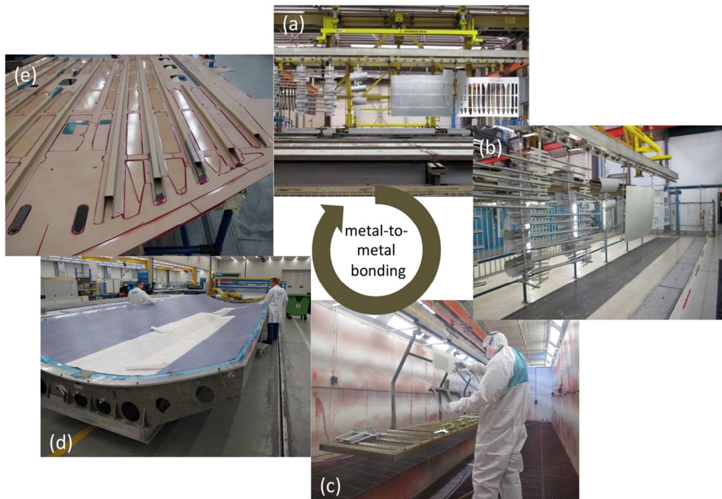
75 Figure 1 The production of metal-to-metal bonding at Fokker Aerostructures: (a) surface pre-treatment (panels hanging 76 above the anodizing bath), (b) parts drying on the rack after pre-treatment, (c) primer application, (d) adhesive application, 77 (e) a bonded part.
