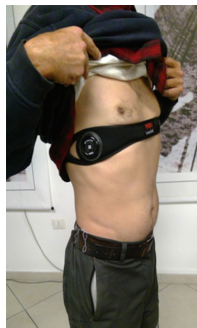
Fig. 4. A worker equipped with Zephyr Bioharness 3
