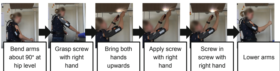
Fig. 3. Individual work steps during the screwing activity with the right hand.
