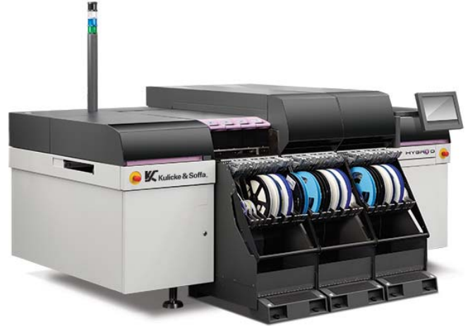
Fig. 12. K&amp;S "Hybrid" with three pick-and-place units.
