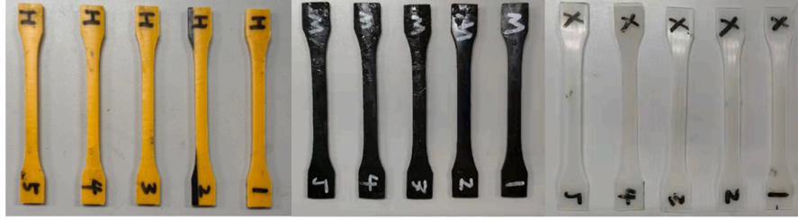
Fig. 10. Dumbbell shape of HDPE (left), MDPE (middle) &amp; XLPE (right).
