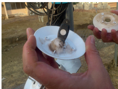
Figure 14: insects in and around moving parts, Ghana
