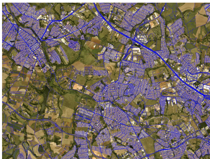
Figure 2.1: Roads detected from Planet satellite imagery 1 .
