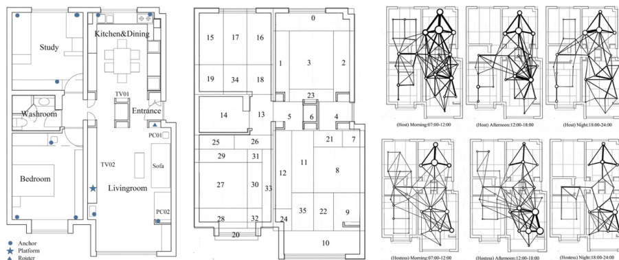
Figure 3.7 : An example of using Indoor positioning devices to track real-time occupation in building (Yang & Huang, 2019).
