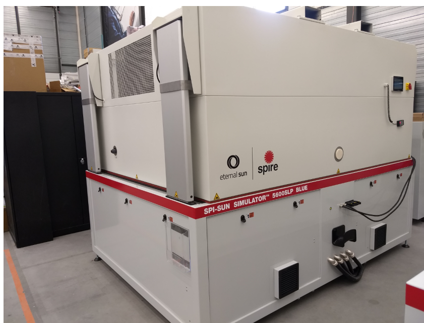
Figure 14: Temperature Controlled Lab Flasher (TCLF) integrating a solar simulator and a temperature chamber, developed by Eternalsun Spire to perform current-voltage measurements at non-standard testing conditions. The temperature chamber can move up, allowing a module to be placed and down to form an insulated environment for heating and cooling.
