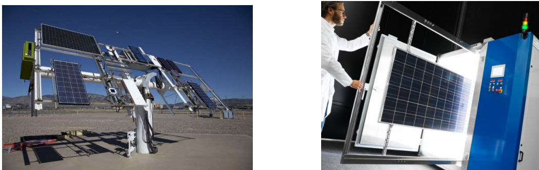
Figure 11: Outdoor (left) and indoor (right) characterization of PV modules. The outdoor setup shows the two-axis tracker installed at Sandia National Laboratories. Figure: Tara Camacho Lopez, 2012, Two-Axis Tracking, accessed 01/16/2020, "https://pvpmc.sandia.gov/modeling-steps/1-weather-design-inputs/array-orientation/two-axis-tracking/" . The indoor setup is a climate chamber integrated continuous solar simulator developed by Eternalsun Spire.
