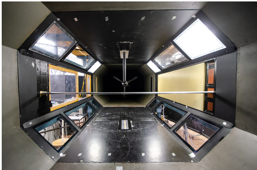
Figure B.2: Front view of the test setup with the wing installed upstream of the propeller in the Low-Turbulence Tunnel at Delft University of Technology
