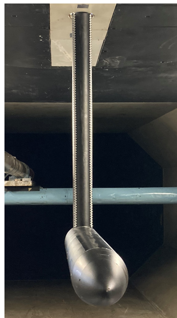
Figure B.5: Photograph showing blade-off configuration including sting and nacelle. The zigzag strips are shown on the sting.
