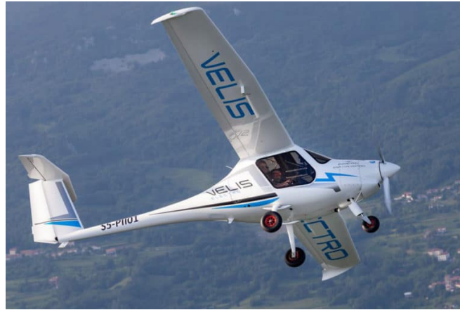
Figure 1.2: Pipistrel Velis Electro, the first EASA-type certified electric aircraft[3]
