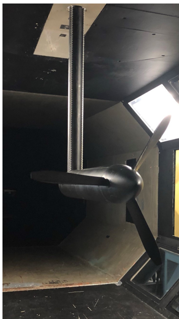
Figure B.4: Photograph of propeller connected to a sting-mounted setup, representing the isolated propeller case
