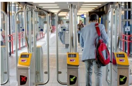
Figure 1, NS Access Control Port (Jacobs, 2016)
