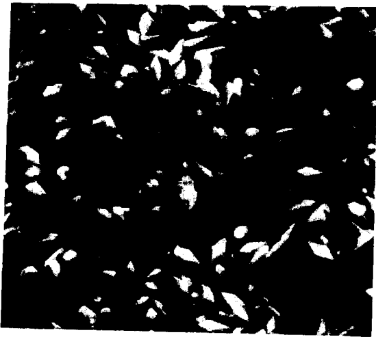
Fig. 4. Scanning electron micrograph of the surface of a titanium nitride layer on molybdenum. The layer is considered to be rough. Deposition conditions: 1100°C, 2% TiCl 4 , H 2 /N 2 =1/1, flow=17 l/h, time=2 h. Bar indicates 5 μm.
