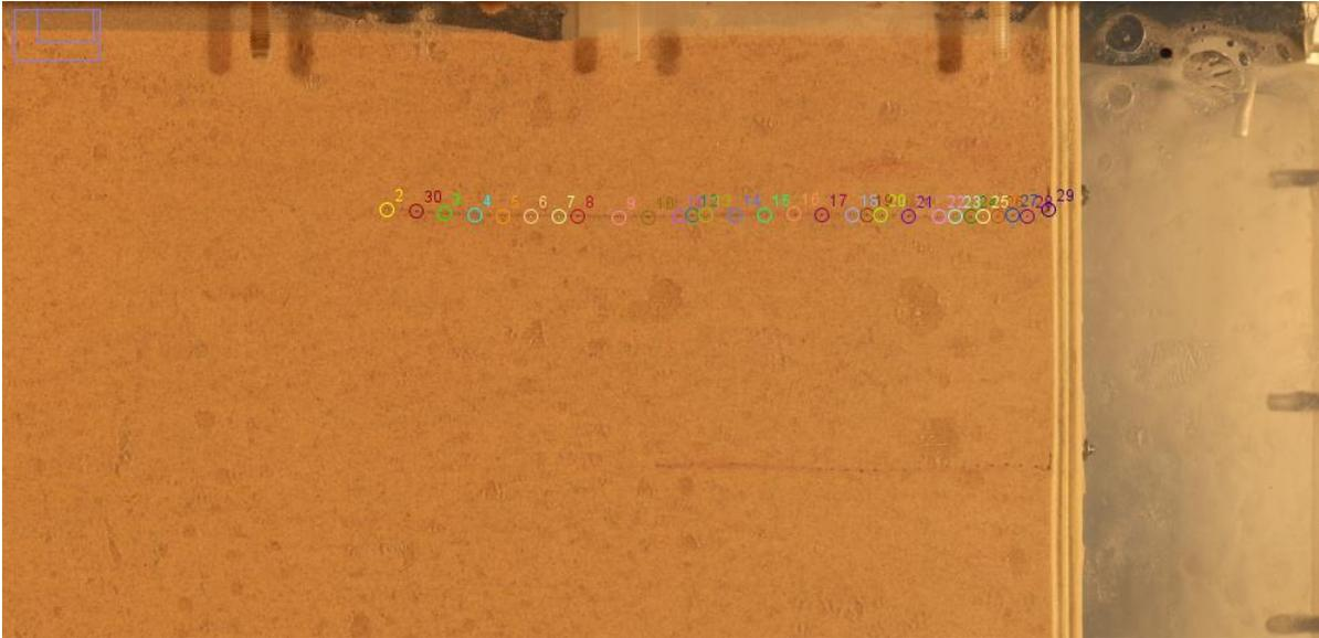
Figure 61: All tracked transverse ribs in order to compute the difference in length between the adjacent ribs and calculate the axial strain. The transverse ribs are ~5 mm apart from each other.
