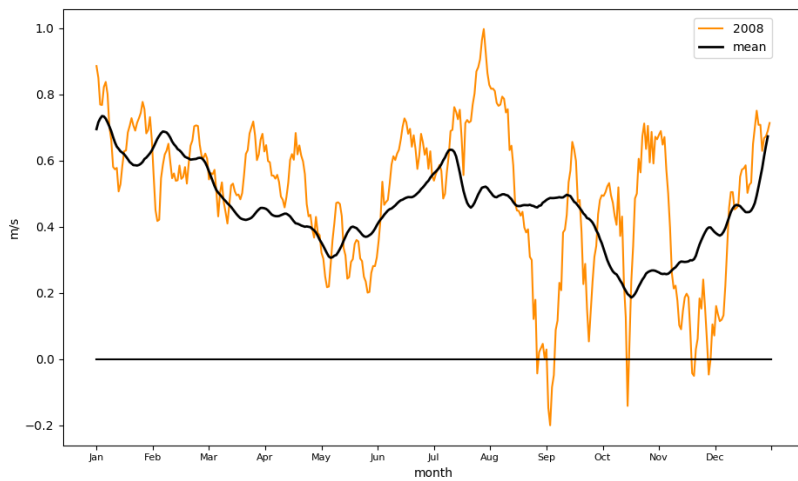
Figure G.2: Surface velocity in the channel region for the year 2008. The black line indicates the mean of all ten years.
