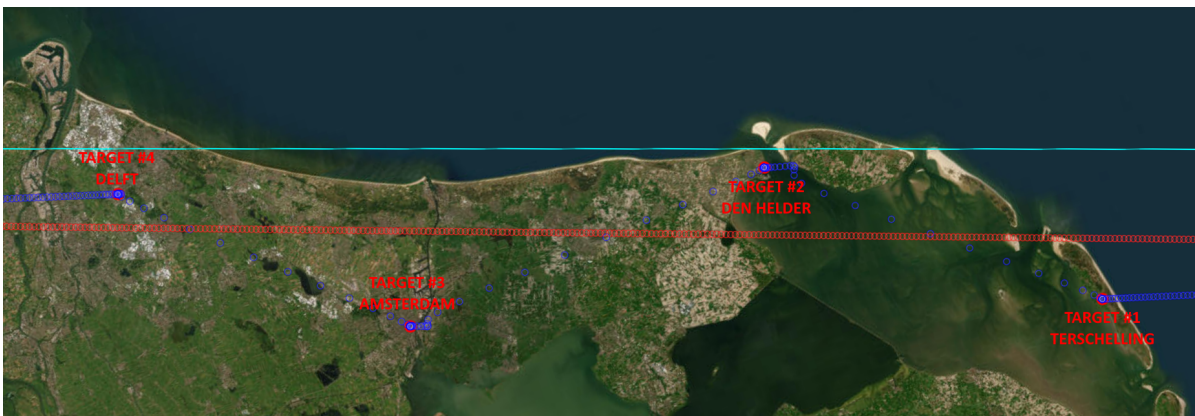
Figure 4.24: Multi-point tracking trajectory. Ground track in cyan, outer loop in red, inner loop in blue.
