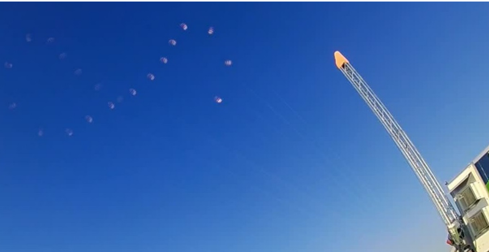
Composite photo of the 20 kN SkySails Power Functional Prototype in crosswind flight
