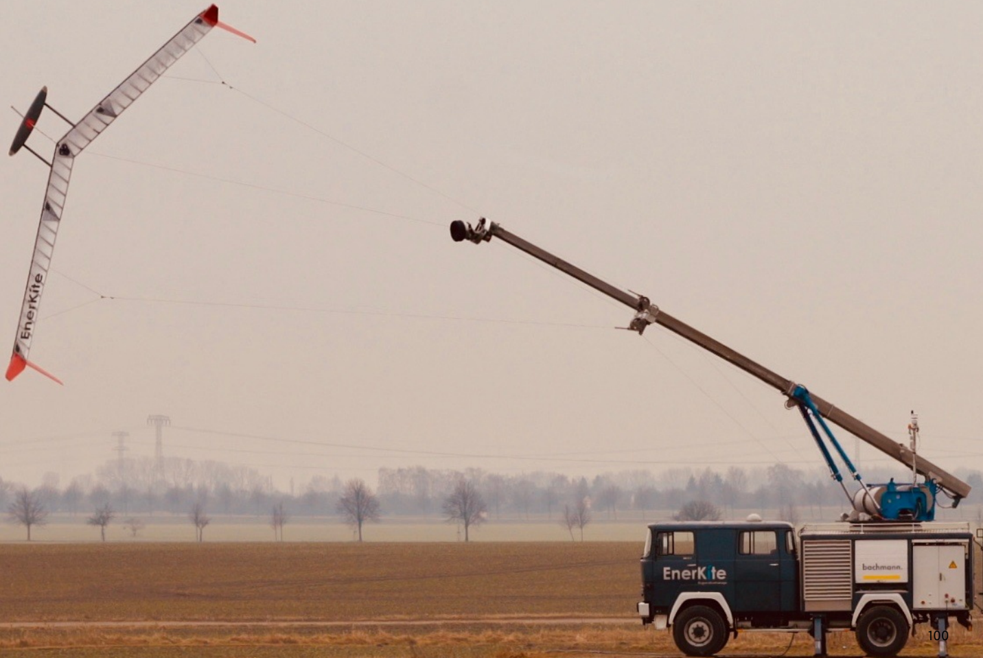
Rotational launch mechanism of Enerkite (25 September 2018)
