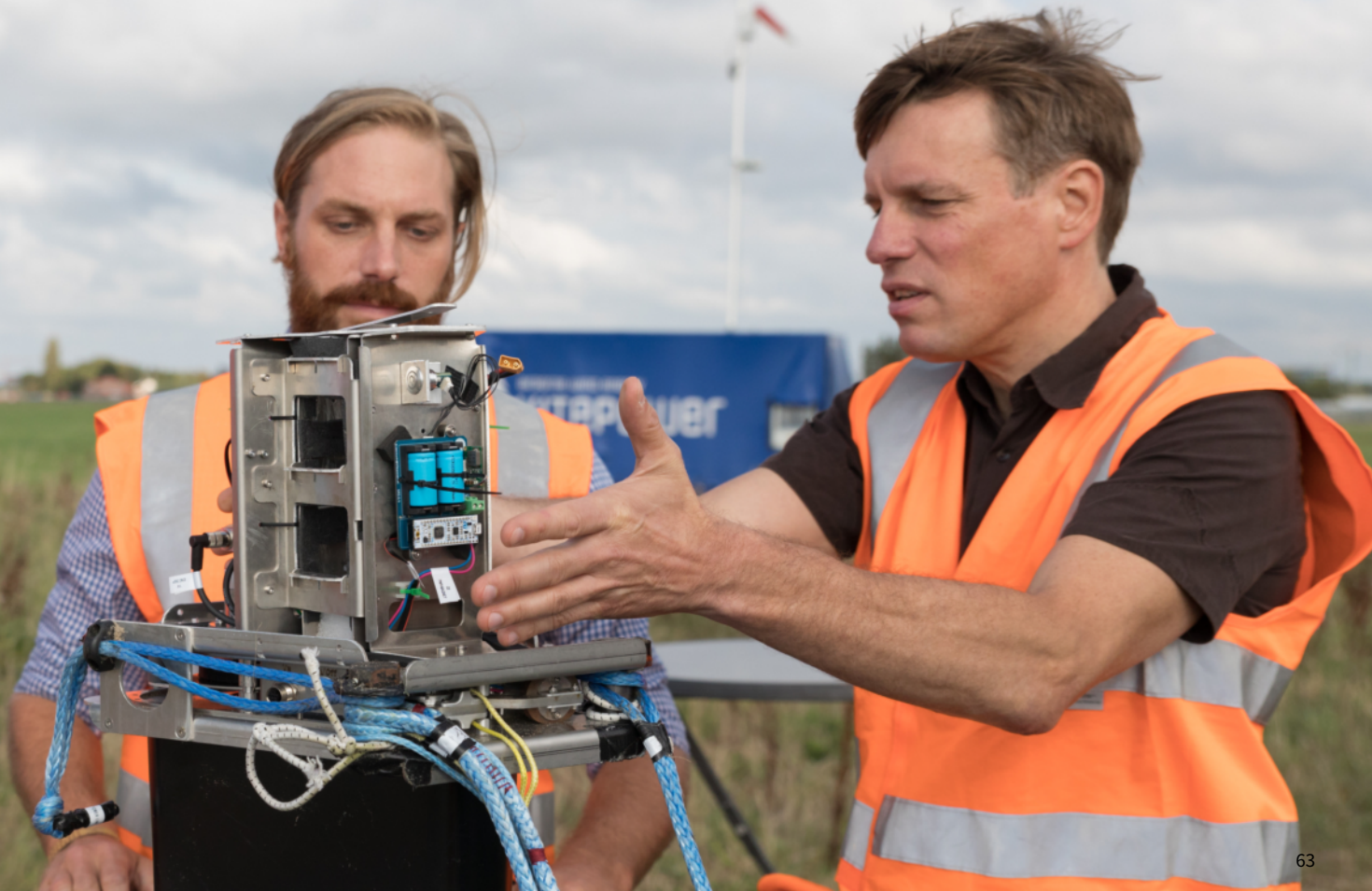
Kitepower co-founders Johannes Peschel (left) and Roland Schmehl (right) explaining a kite control unit (29 August 2019)
