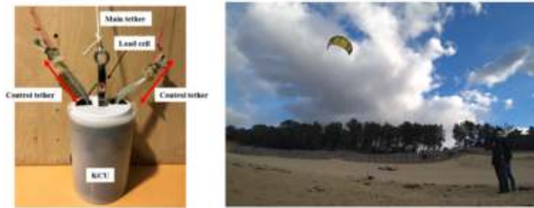
Figure 1: Kite power system: KCU, and Real Flight Test.
