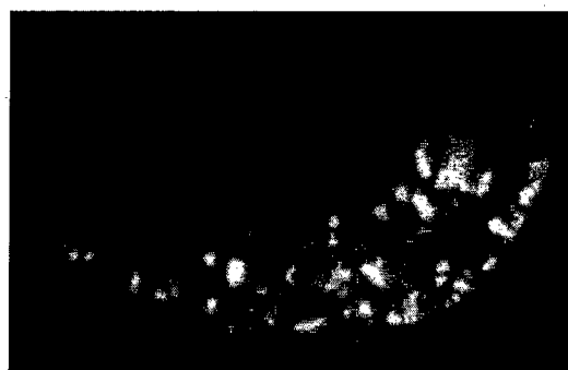
Figure 15: OH emission of HNF C15 / GAP propellant at 0.15 MPa (image size = 4.1 \times 6.2 \text{ mm}^2 ).
