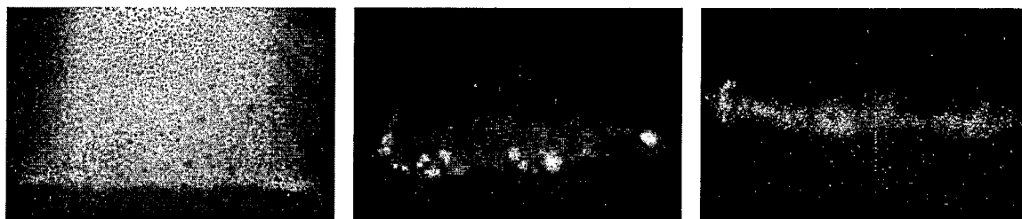
Figure 14: OH emission at 0.3 MPa. From left to right: HNF, HNF C15 / GAP and HNF S16 / GAP. (image size 4.1 \times 6.2 \text{ mm}^2 )
