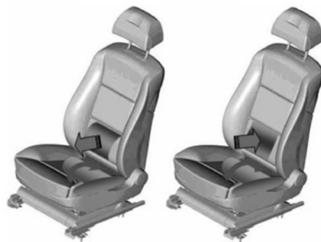
Fig. 11 Roll function of lumbar support (Franz, 2010).
