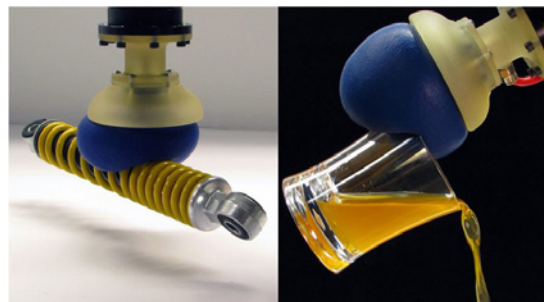
Fig. 62 Gripper by Brown et al. (2010) in use.
