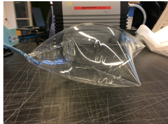
Fig. 73 Foam embedded in the actuator. When actuated, the inflatable behaves alike the one without foam inside because the foam is not glued to the external surfaces of the chamber.
