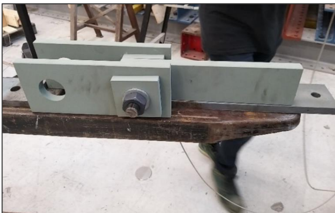
Figure 5.6 - Left) Specimen assembly; Right) Preloading of the bolts
