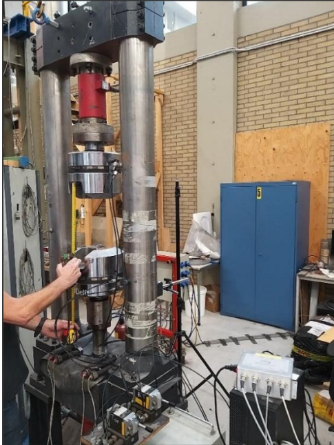
Figure 5.5 - Setting up the Dowty Rotel cyclic loading machine
