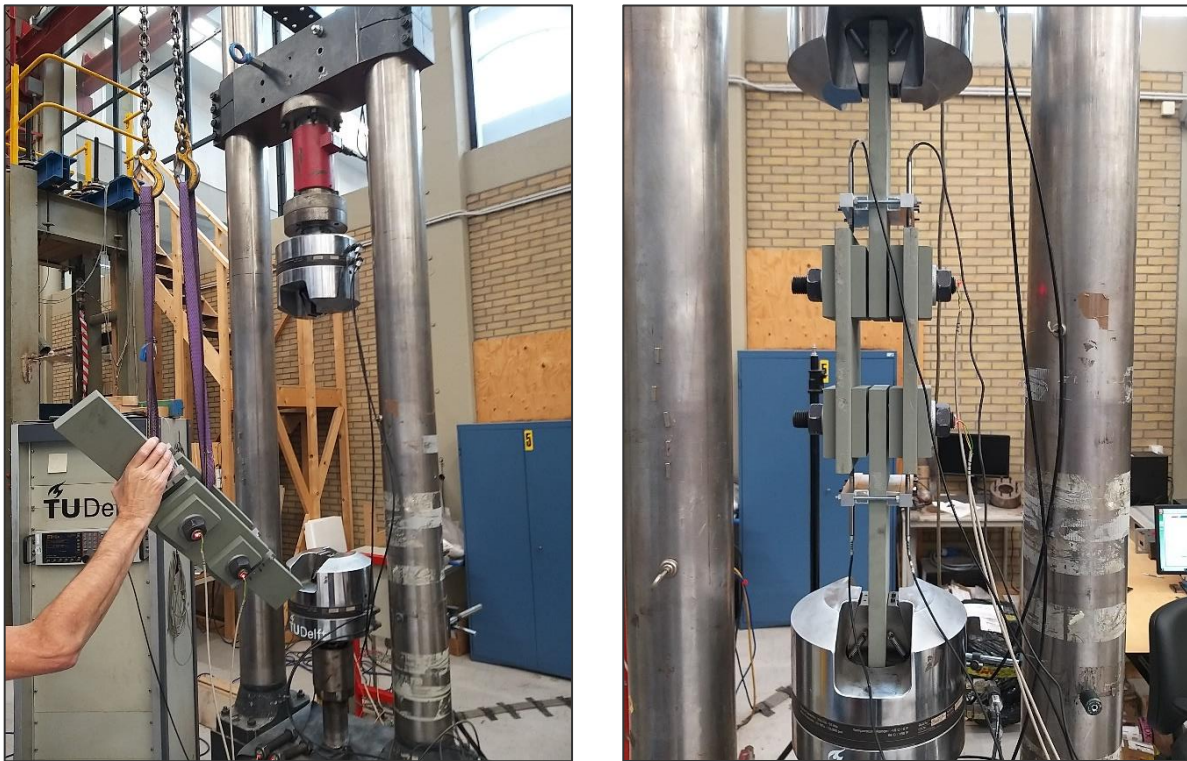
Figure 5.7 - Left) Moving the specimen; Right) Specimen placed in cyclic loading machine
