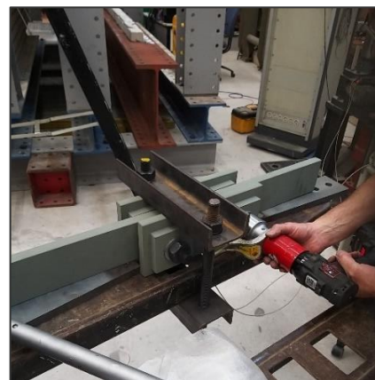
Figure 5.6 - Left) Specimen assembly; Right) Preloading of the bolts
