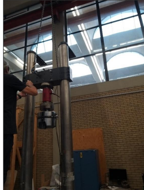
Figure 5.5 - Setting up the Dowty Rotel cyclic loading machine
