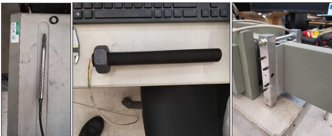
Figure 5.4 - Left) LVDT; Middle) Strain bolt; Right) LVDT support assembly
