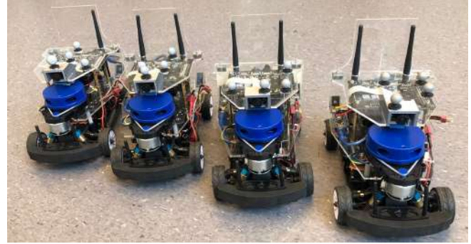
Fig. 1: DART, a small-scale robotic platform for autonomous driving research.
