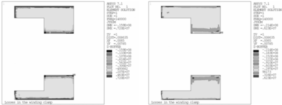
Figure C.11. The real (left) and imaginary (right) component of the current density in the aluminium heat sink
