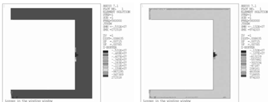
Figure C.8. The real (left) and imaginary (right) component of the current density in the aluminium heat sink
