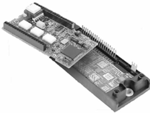
The I 2 PM with integrated gate drives, protection and controller (Source: International Rectifier)
