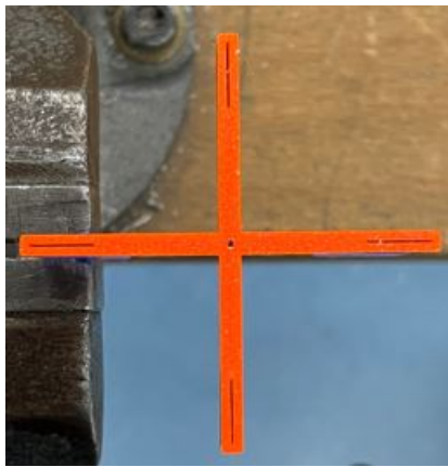
Figure A.5: Slits for the leaf spring flexures and the whole through which the SMA wire is inserted.
