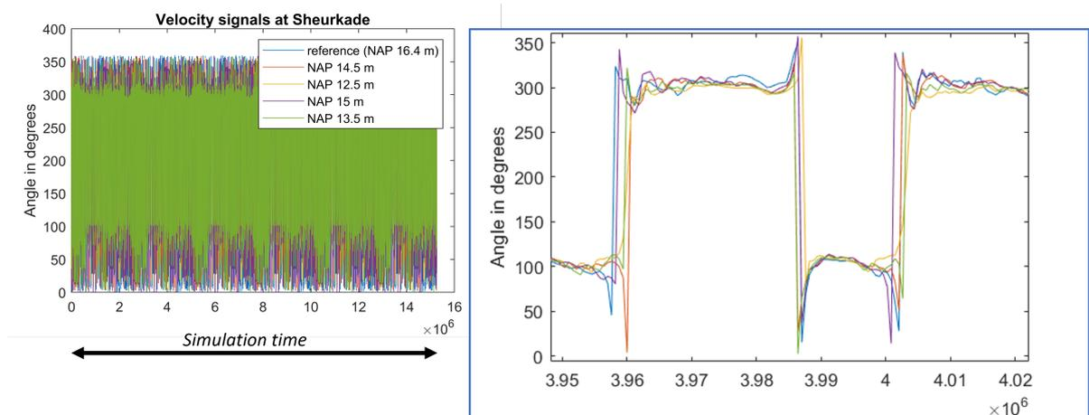
Figure C.5: Left: Velocity angle time series used in the OpenTNSim model. The hydrodynamic conditions for each state (reference and shallowing) were obtained from the OSR model. Right: Extension over slightly more than one tidal period. Non systematic difference can be observed when comparing different shallowing levels.
