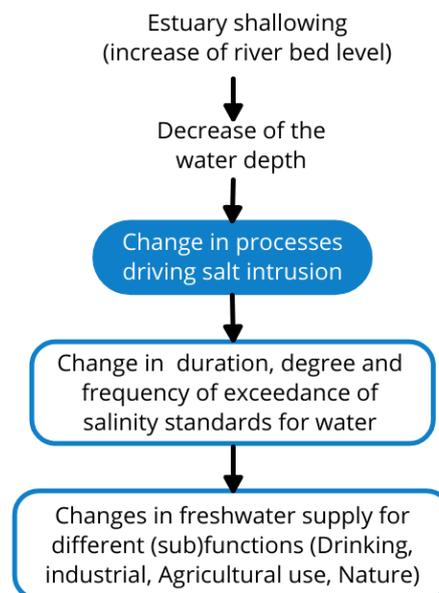
Figure 2.4: Framework for the assessment of implications of shallowing on freshwater supply.
