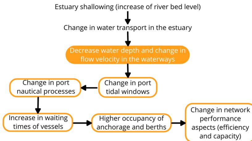
Figure 2.9: Framework for the assessment of implications of shallowing on port efficiency and capacity.
