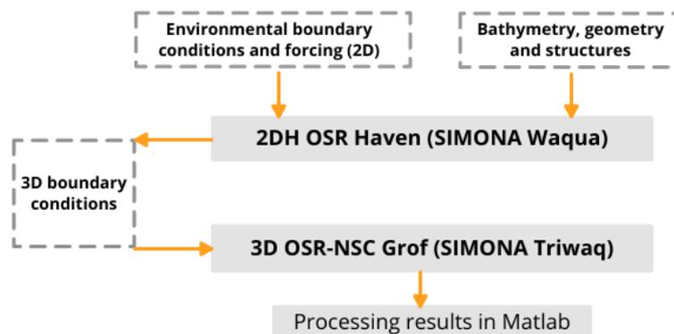
Figure 3.8: Overview of the structure of the OSR model.
