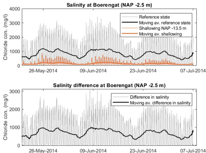
Figure B.24: Impact of shallowing NAP -12.5 m on chloride concentration at Boerengat. Values are computed at a water depth of approximately NAP -2.5 m, since this is the water inlet suction depth. The figure shows the 10 min time step signal for the reference and shallowing state, and the corresponding moving averages calculated over two tides (24.8 hs).
