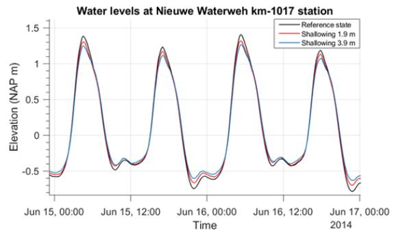
Figure B.12: Left: Time series of the water level computed at the controlling station on the Nieuwe Waterweg km-1017, for different bed levels. The simulation was conducted for a period without wind set-up. The total simulation time is 42 days. Right: The figure shows an expansion of the time series for the period between the 15-06 and 17-06.
