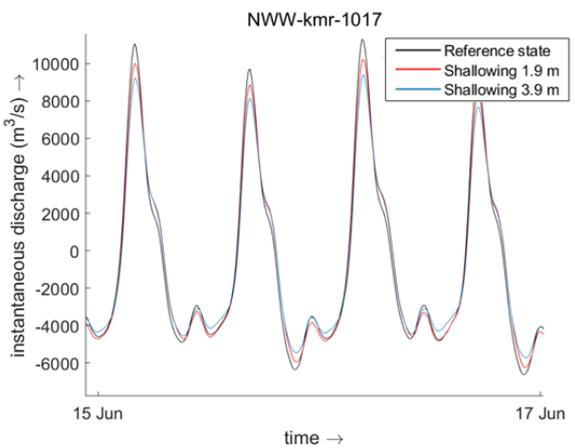
Figure B.13: Left: Time series of the tidal flow discharge amplitude computed at the controlling station on the Nieuwe Waterweg km-1017, for different bed levels. Right: The figure shows an expansion of the time series for the period between the 15-06 and 17-06.
