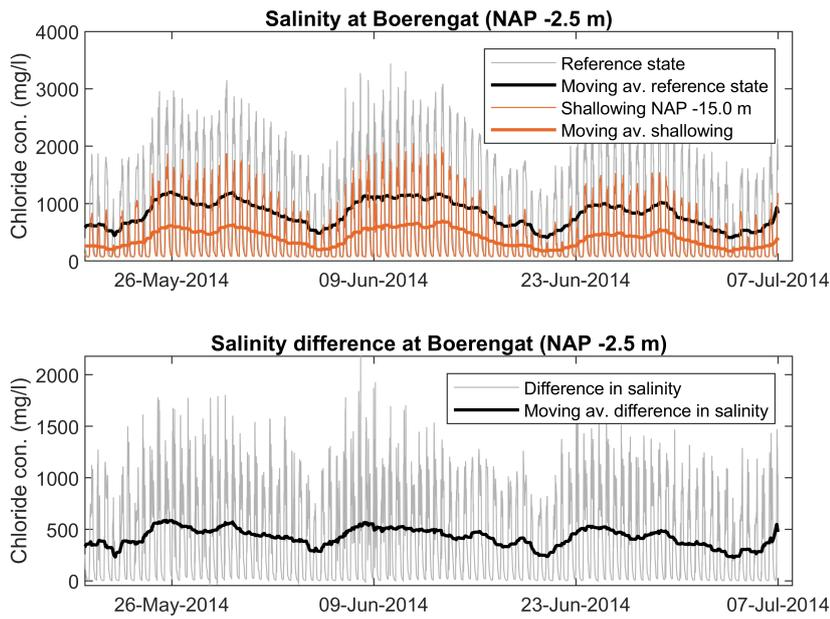
Figure B.21: Impact of shallowing NAP -15.0 m on chloride concentration at Boerengat. Values are computed at a water depth of approximately NAP -2.5 m, since this is the water inlet suction depth. The figure shows the 10 min time step signal for the reference and shallowing state, and the corresponding moving averages calculated over two tides (24.8 hs).
