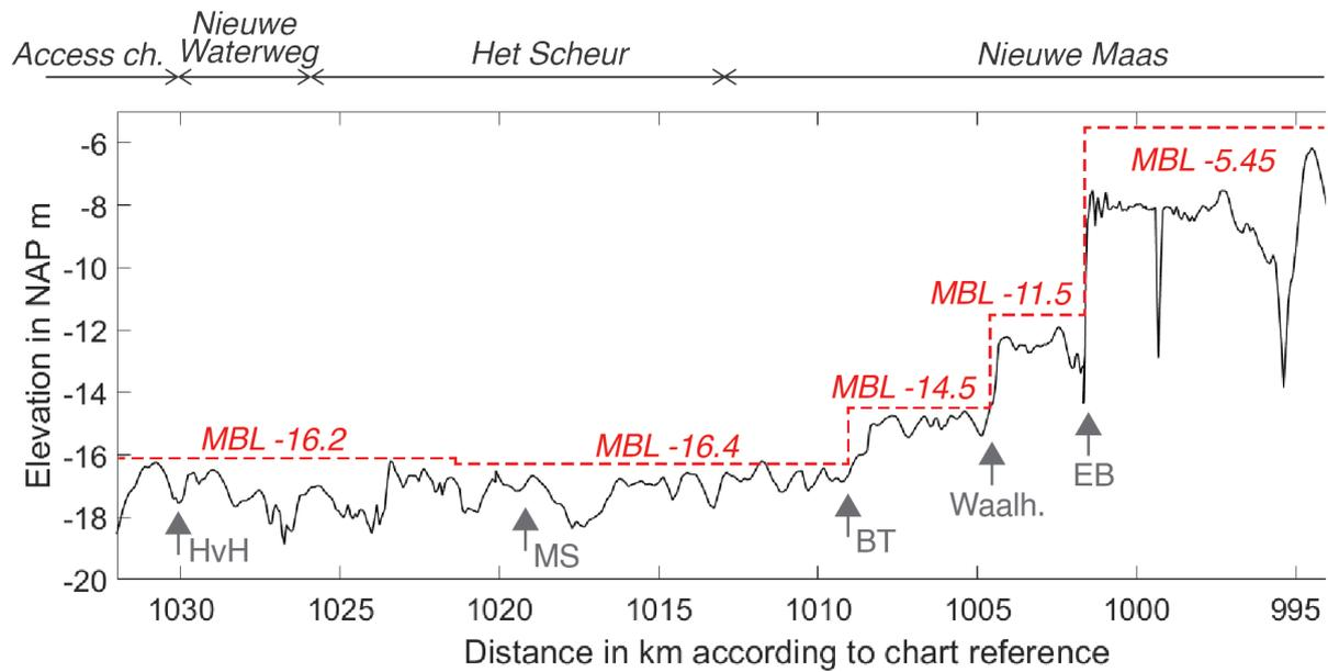
Figure 3.4: River bottom bathymetry in the Rotterdam Waterways. The figure shows, in dashed red line, the Maintained Bed Level (MBL) along the Nieuwe Waterweg and Nieuwe Maas, according to the harbour chart of the PoR [Port of Rotterdam Authority, 2021]. Also, the actual bed level is depicted in black solid line.
