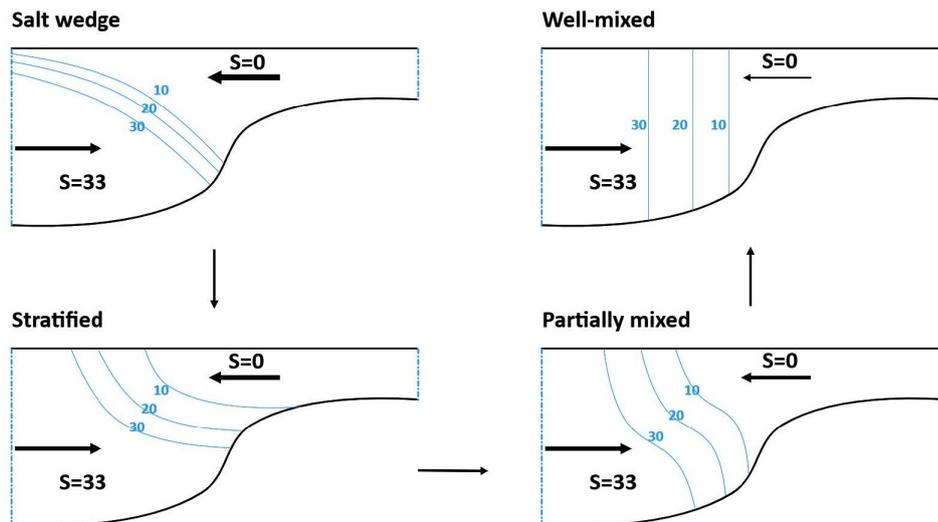
Figure 2.2: Types of estuaries based on degree of salt-fresh mixing. Numbers denote salinity in Practical Salinity Units [PSU] [Pietrzak, 2020]
