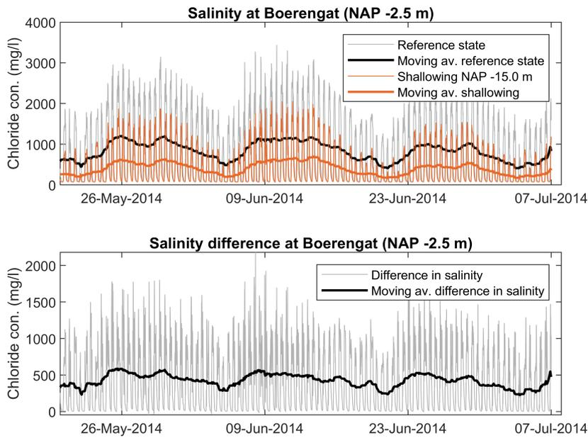
Figure B.22: Impact of shallowing NAP -14.5 m on chloride concentration at Boerengat. Values are computed at a water depth of approximately NAP -2.5 m, since this is the water inlet suction depth. The figure shows the 10 min time step signal for the reference and shallowing state, and the corresponding moving averages calculated over two tides (24.8 hs).
