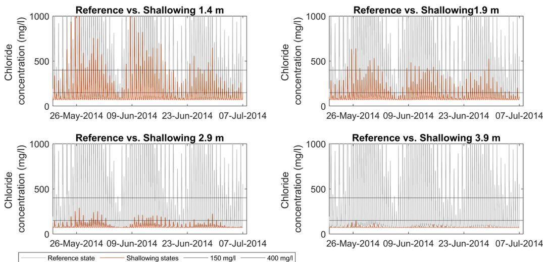
Figure 4.4: Impact of shallowing on the chloride concentration at Brienoordbrug. The figure presents the time series of for the reference case (grey lines in the background) and the shallowing states (orange lines). The two horizontal lines correspond to the 150 mg/l and 400 mg/l thresholds for drinking and agricultural water use, respectively.
