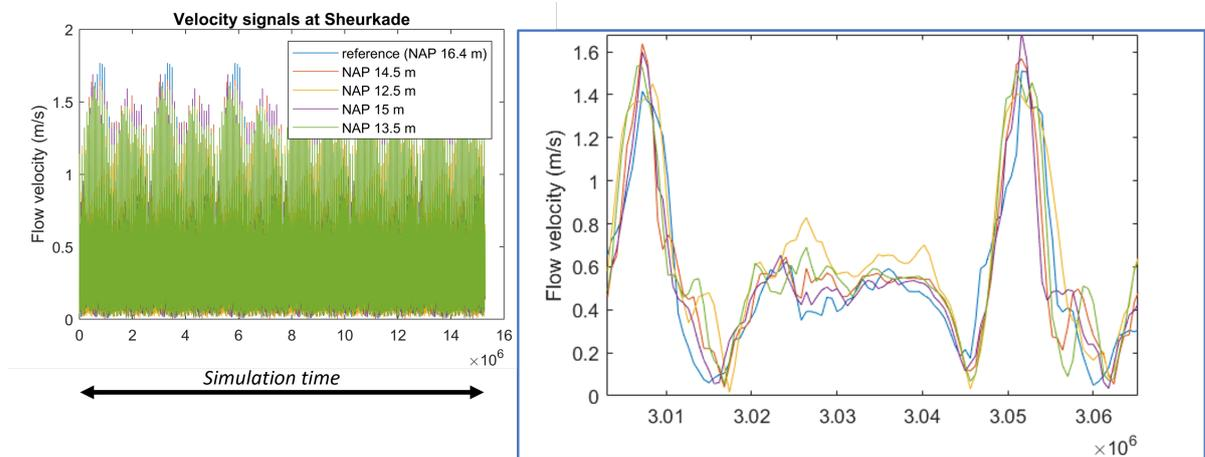
Figure C.4: Left: Velocity magnitude time series used in the OpenTNSim model. The hydrodynamic conditions for each state (reference and shallowing) were obtained from the OSR model. Right: Extension over slightly more than one tidal period. In this figure, a slight increase in flow velocity magnitude is not completely visible. To have better insights on the effect of shallowing on velocity magnitudes, the reader is referred to Figure B.7.
