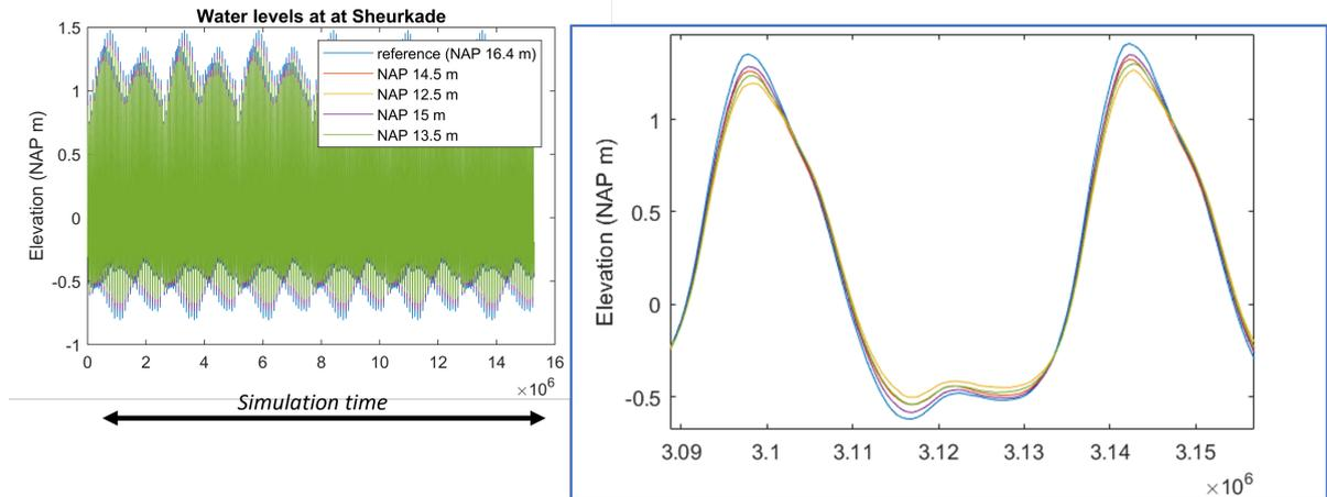
Figure C.3: Left: Water level time series used in the OpenTNSim model. The hydrodynamic conditions for each state (reference and shallowing) were obtained from the OSR model. Right: Extension over slightly more than one tidal period. In this figure, a slight decrease in the tidal range is visible.
