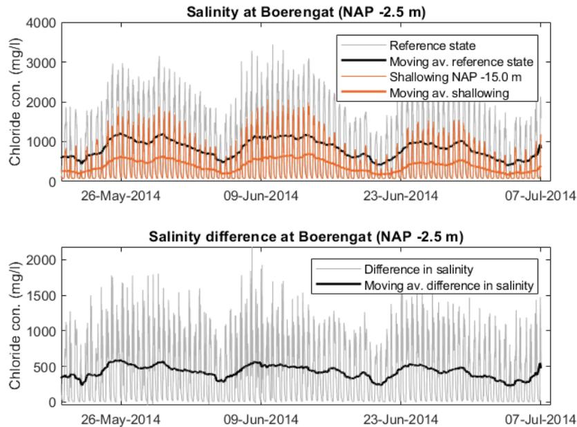
Figure B.23: Impact of shallowing NAP -15.0 m on chloride concentration at Boerengat. Values are computed at a water depth of approximately NAP -2.5 m, since this is the water inlet suction depth. The figure shows the 10 min time step signal for the reference and shallowing state, and the corresponding moving averages calculated over two tides (24.8 hs).
