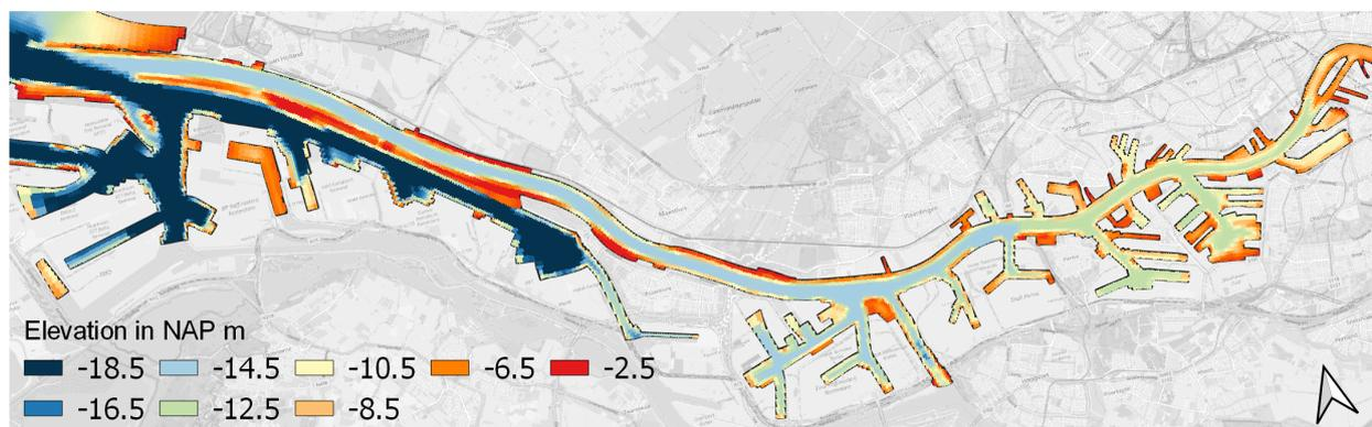
Figure B.3: Bathymetry for the shallowing up to NAP -14.5 m. Shallowed areas are depicted in dark blue. The colour bar of this figure was adjusted so that shallowed areas can easily be viewed.
