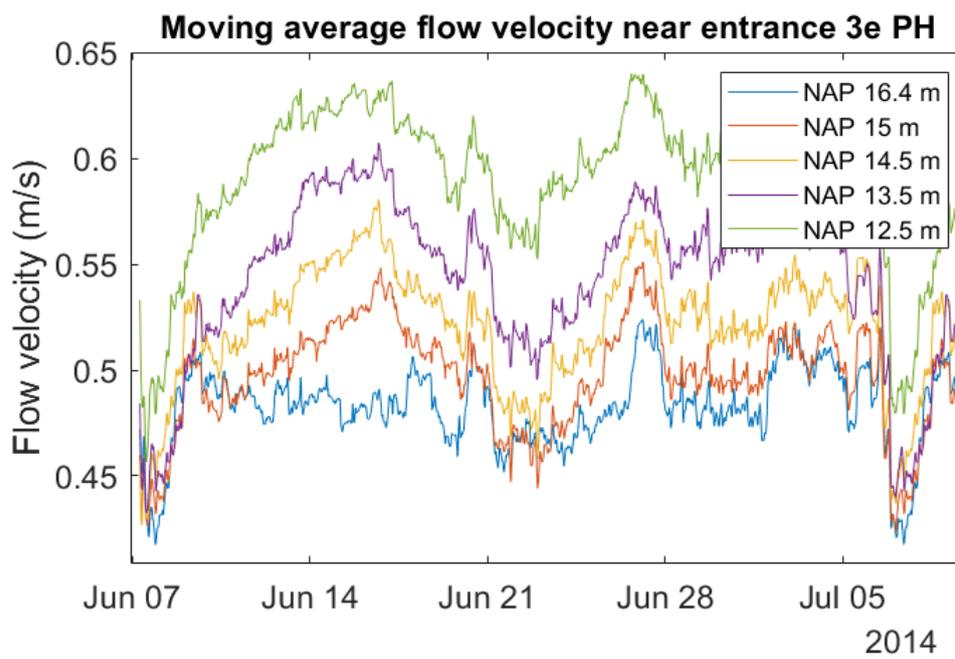
Figure C.6: Moving average of flow velocities calculated over two tidal periods (24.8 hs). The figure presents outcomes for all levels of shallowing, computed at the entrance of the 3e Petroleumhaven (Node 15 in the network).
