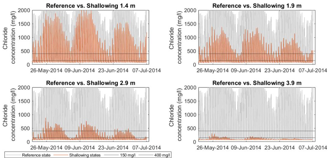
Figure 4.3: Impact of shallowing on the chloride concentration at the Boerengat water inlet. The figure presents the salinity time series at the water inlet for the reference case (grey lines in the background) and the shallowing states (orange lines). The two horizontal lines correspond to the 150 mg/l and 400 mg/l thresholds for drinking and agricultural water use, respectively.
