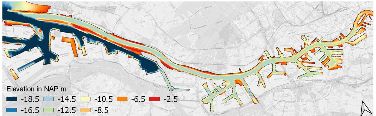
Figure B.4: Bathymetry for the shallowing up to NAP -13.5 m. Shallowed areas are depicted in dark blue. The colour bar of this figure was adjusted so that shallowed areas can easily be viewed.
