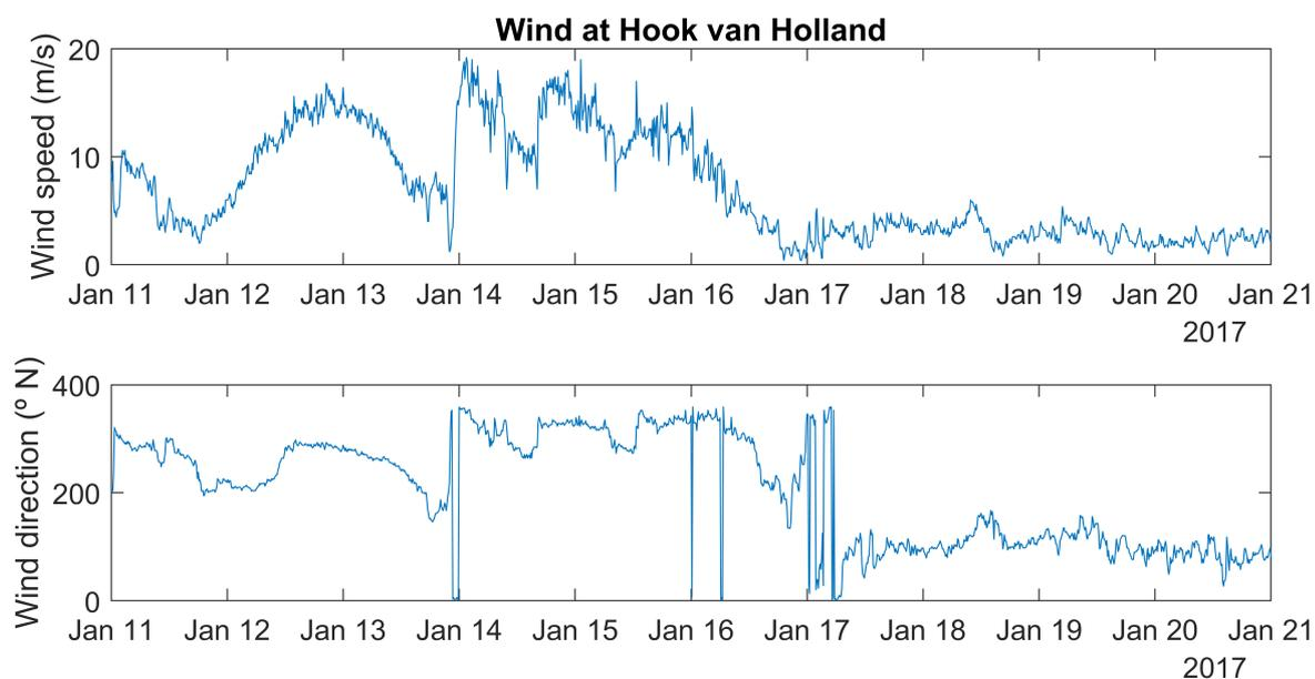
Figure B.25: Wind forcing used in the OSR-model for the simulations described in Section B.1.4. The upper plot shows the wind direction, and the lower plot presents the wind speed. As seen from the figure, high wind speeds over 10 m/s are present between the 12th and 16th of January.
