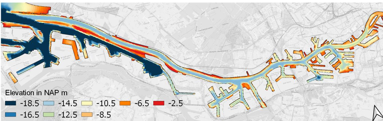
Figure B.2: Bathymetry for the shallowing up to NAP -15.0 m. Shallowed areas are depicted in dark blue. The colour bar of this figure was adjusted so that shallowed areas can easily be viewed.
