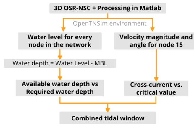
Figure 3.14: Overview structure of the tidal window calculation (see also Appendix C) for an exemplar illustration of the calculation.
