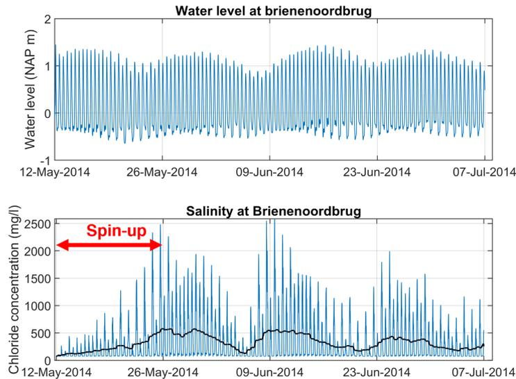
Figure B.9: Chloride content time series obtained with the OSR model at Brienenoordbrug. The time series corresponds to the reference case. The figure shows the 10 min time step signal in blue and the moving average calculated over two tides (24.8 hs) in black. The spin-up time is estimated from the 12-05 until the 26-05.
