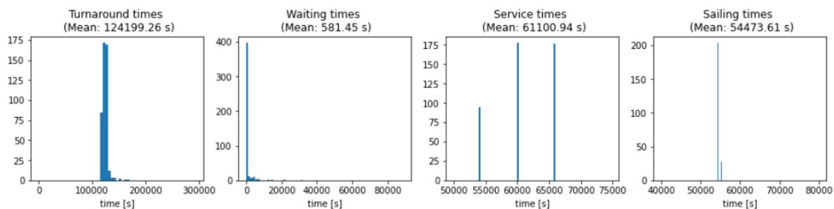
Figure C.8: OpenTNSim model results for the shallowing 1 state. Waiting times, turnaround times and service times distributions for Run 1.
