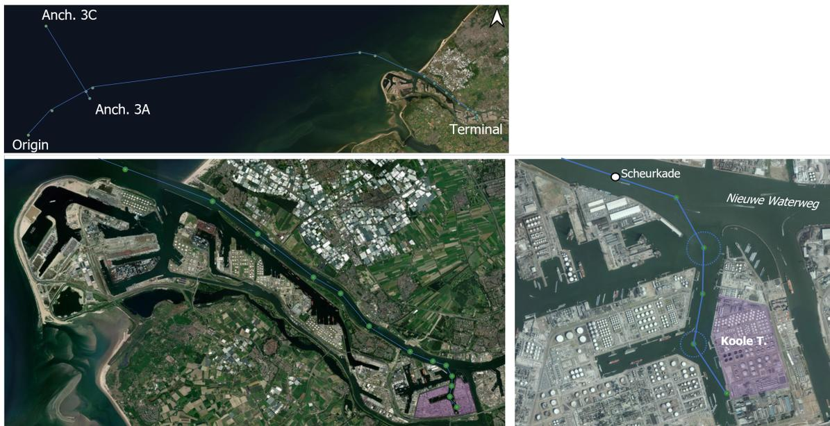
Figure 3.12: Port and waterways system network, boundaries and components. The route is depicted in blue, with green dots representing nodes. Turning basins in the lower right map are depicted in blue dashed line. The purple area in the lower-left map represents the 3rd Petroleum Haven area, whereas the lower right map represents the Koole liquid bulk terminal.
