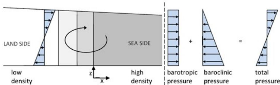
Figure 2.3: Vertical distribution of pressures resulting in the total pressure forcing estuarine circulation [Pietrzak, 2020]. The barotropic pressure is seaward directed, whereas the baroclinic pressure is directed up estuary. The resulting pressure leads to a circulatory flow pattern in which the upper part of the flow is forced seawards while the lower part is driven landwards.
