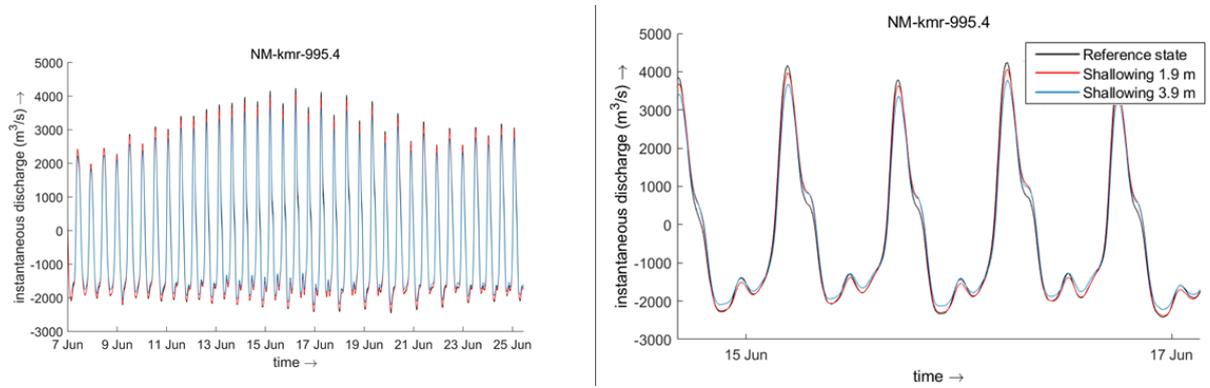
Figure B.14: Left: Time series of the tidal flow discharge amplitude computed at the controlling station on the Nieuwe Maas km-995, for different bed levels. Right: The figure shows an expansion of the time series for the period between the 15-06 and 17-06.
