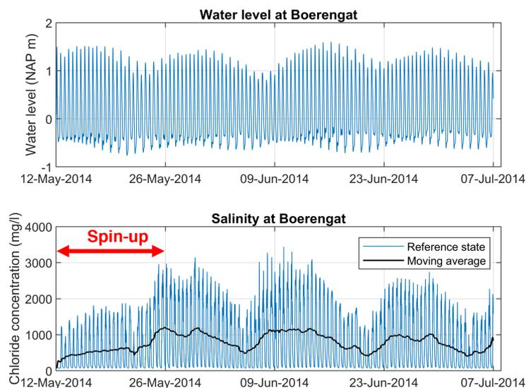
Figure B.8: Chloride content time series obtained with the OSR model at the Boerengat water inlet. The time series corresponds to the reference case. The figure shows the 10 min time step signal in blue and the moving average calculated over two tides (24.8) in black. The spin-up time is estimated from the 12-05 until the 26-05.
