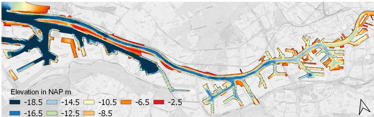
Figure B.1: Bathymetry for the reference state.
