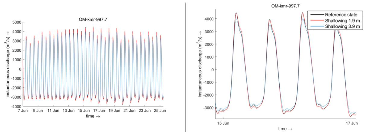
Figure B.15: Left: Time series of the tidal flow discharge amplitude computed at the controlling station on the Oude Maas km-997, for different bed levels. Right: The figure shows an expansion of the time series for the period between the 15-06 and 17-06.
