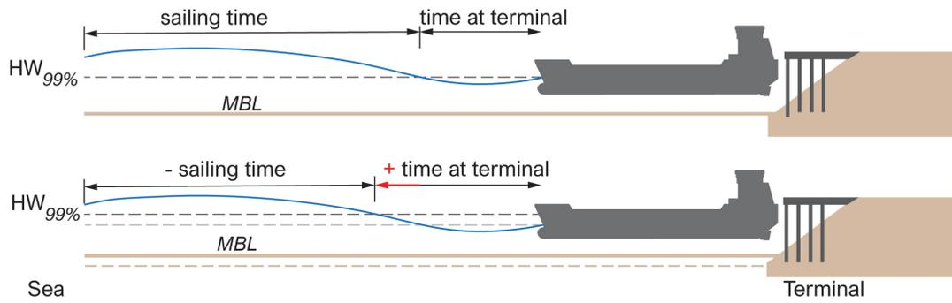
Figure 2.8: Effect of estuary shallowing on waiting times for an outbound vessel. The figure represents a typical seagoing vessel leaving the terminal. The situation is analogous to the one presented in Figure 2.7. In this case, shallowing leads to longer waiting times of vessels at the terminal trying to depart.
