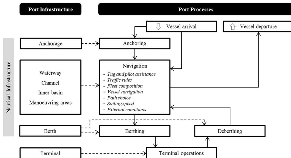
Figure 2.5: Diagram of port nautical infrastructure and processes according to Olba et al. [2018].
