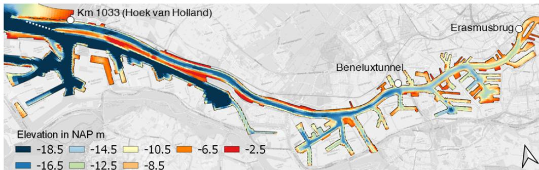
Figure 3.10: Bathymetry map for the reference state. All areas deeper than NAP -18 m are depicted in dark blue. As seen from this figure, the actual depth of the river section between Hoek van Holland and the Beneluxtunnel is generally between NAP -16 m and NAP -18 m.
