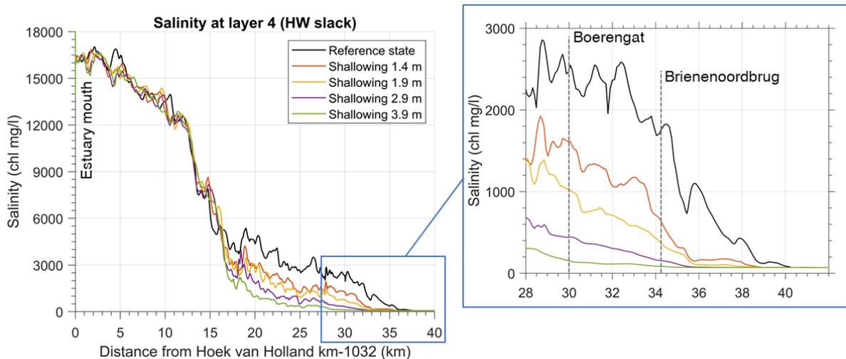
Figure 4.2: Chloride content along the Nieuwe Waterweg and Nieuwe Maas, during high slack water and neap tide. The figure shows longitudinal salinity variation on the 24-06 at 16 hs. The longitudinal transect crosses through the centre of the river cross-section at 46% of the water depth (around NAP -2.5 m, and assumed to be the water suction depth). Although it is not the most extreme case in the simulation, this situation corresponds to a typical salinity peak during low mixing conditions.
