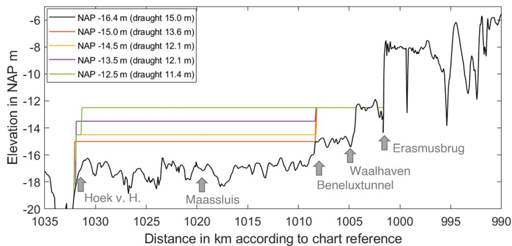
Figure 3.6: Bed levels along the Nieuwe Waterway and Nieuwe Maas for a longitudinal transect through the channel center. The reference state (black line) and shallowing bed levels (coloured lines) are depicted. Bathymetry values for the reference state (black line) were provided by the Port of Rotterdam Authority. The legend indicates the design vessel draught that corresponds to each shallowing state.
