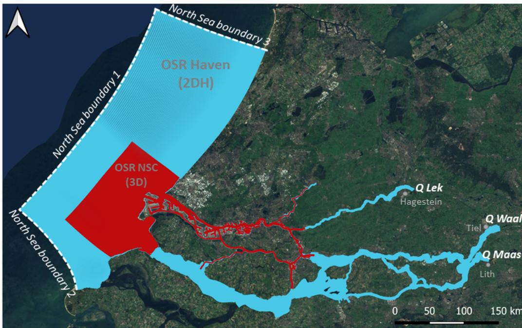
Figure 3.7: Boundary conditions of the OSR model. The 2DH OSR Haven model (cyan colour) nests the 3D OSR NSC model (red colour). Conditions are imposed at three sea boundaries and three river boundaries, from which the new boundary conditions for the 3D model are derived. Bathymetry changes are implemented to both models.
