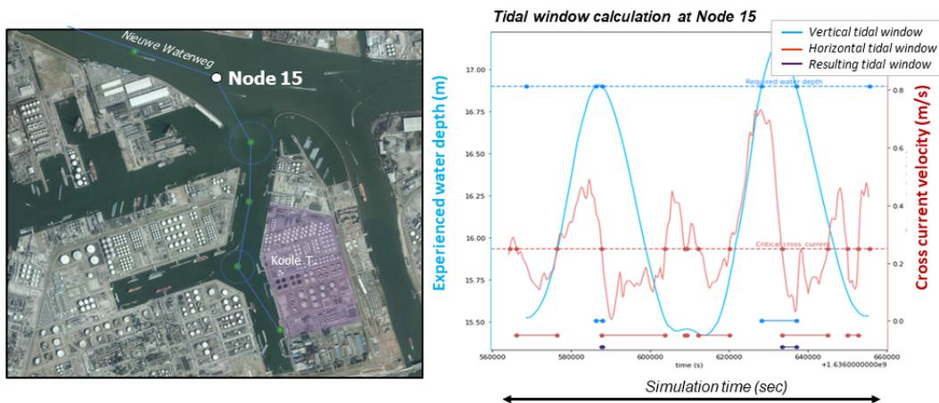
Figure C.2: Tidal window calculation. The right figure details the model network at the 3rd Petroleumhaven basin and Koole terminal. The left figure presents combined tidal window at node 15 as calculated by the model. The available tidal window results from overlapping the vertical and horizontal tidal windows.
