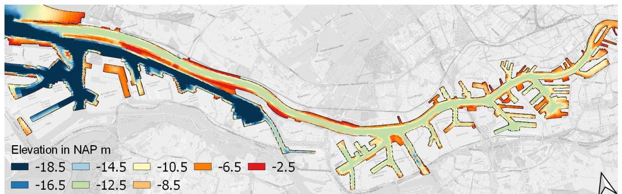
Figure B.5: Bathymetry for the shallowing up to NAP -12.5 m. Shallowed areas are depicted in dark blue. The colour bar of this figure was adjusted so that shallowed areas can easily be viewed.
