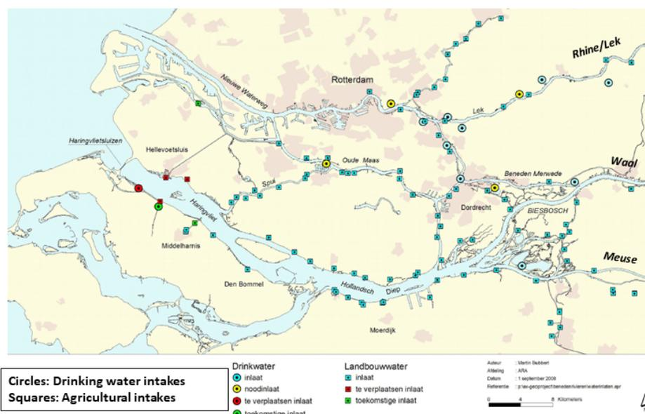
Figure A.1: Map of the freshwater supply system in the Rhine-Meuse Delta (from Rijkswaterstaat).
