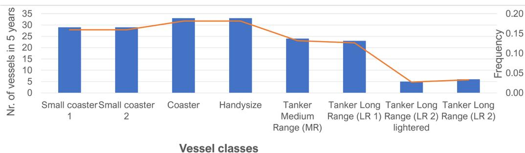
Figure 3.13: Fleet size distribution assumed for the Koole terminal in the 3rd Petroleum Haven. The x-axis shows the vessel classes used in the modelling study. The y-axis on the left shows arrivals at the Koole terminal between January 2015 and February 2020 from de Jong [2020]. The number of vessels for coasters and small coasters was assumed. The y-axis on the right and the orange line present the relative frequency of arrivals, based on the number of arrivals.
