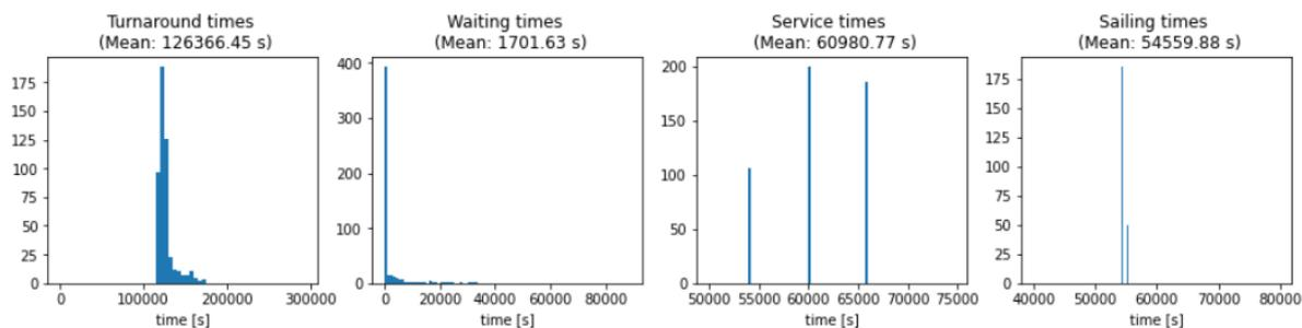
Figure C.10: OpenTNSim model results for the shallowing 3 state. Waiting times, turnaround times and service times distributions for Run 1.
