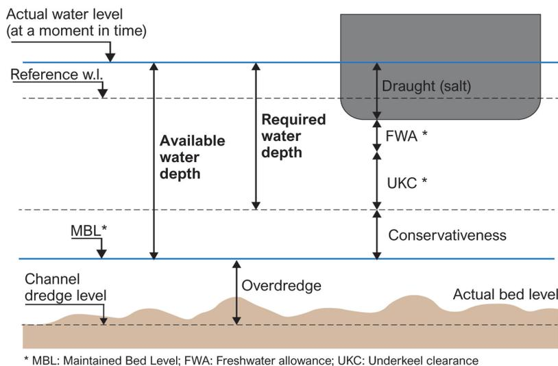
Figure 2.6: Relevant parameters in vertical design of vessels. In particular, the figure sketches the available and required water depth at a moment in time (image modified from de Jong [2020]).
