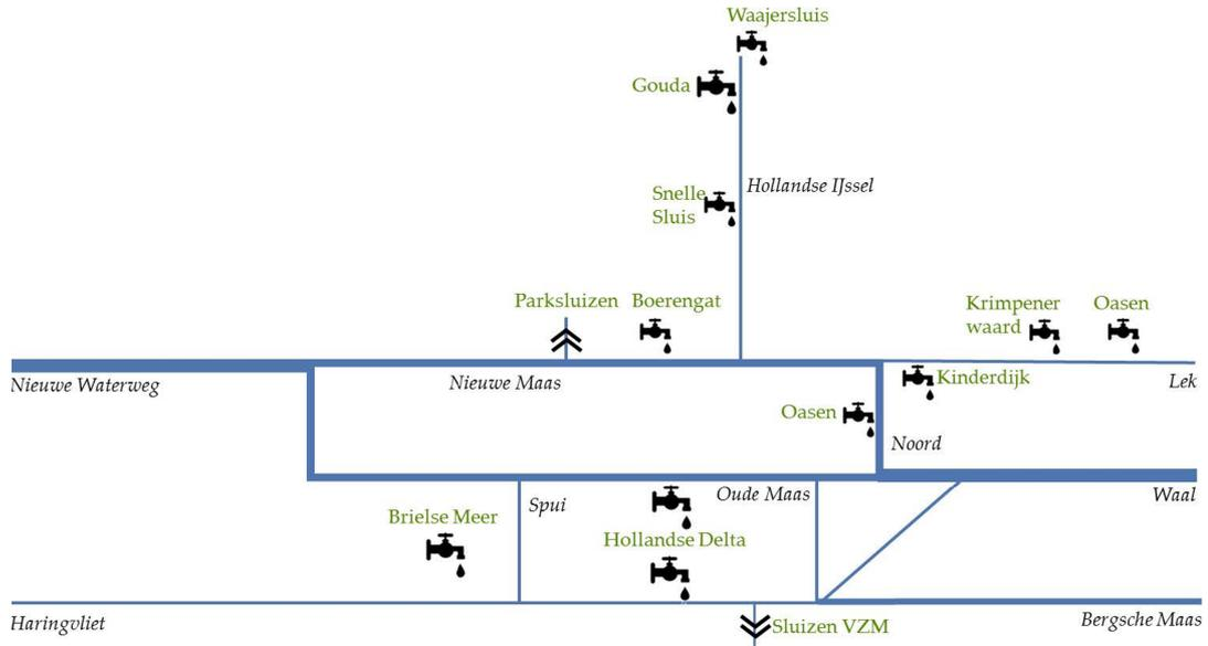
Figure A.2: Schematization of the freshwater supply system in the RMD with the most important water inlets [Hydrologic, 2015]. The thickness of the blue lines is proportional to the discharge distribution during a period of low river run-off i.e. when flow rate measured at Lobith is below 1500 m<sup>3</sup>/s).
