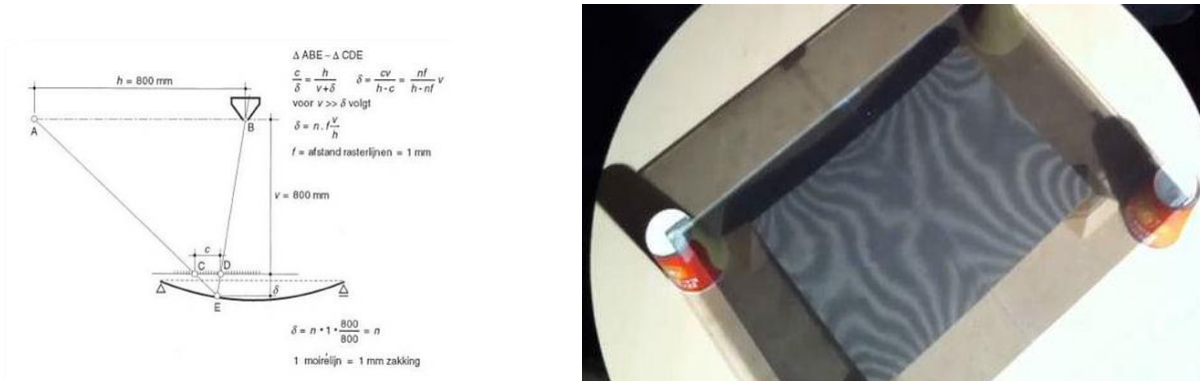
Fig.11: Moiré patterns showing deflections of an out-of-plane loaded plate
