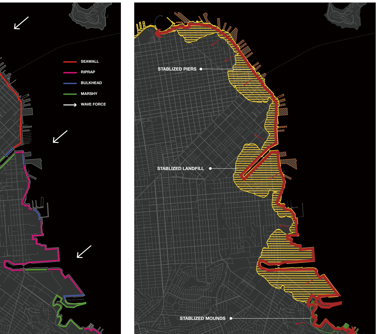
Fig.27: Stabilization. Drawed by Author.
