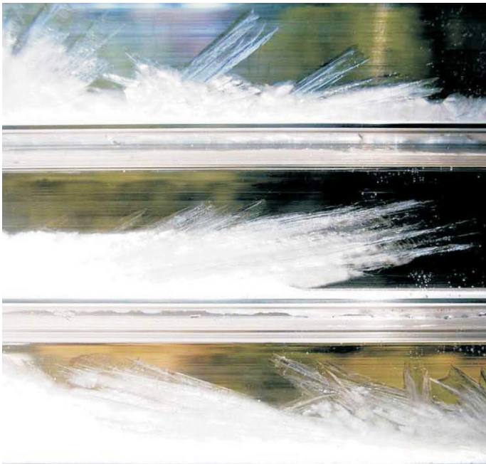
FIG. 5 - Glass pane with embedded PCM in its changing state
