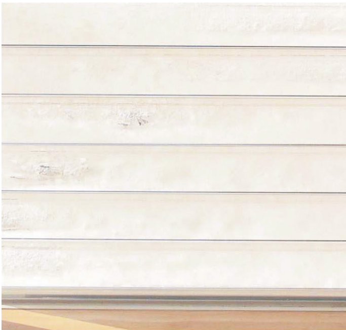
FIG. 6 - Glass pane with embedded PCM in its crystal state
