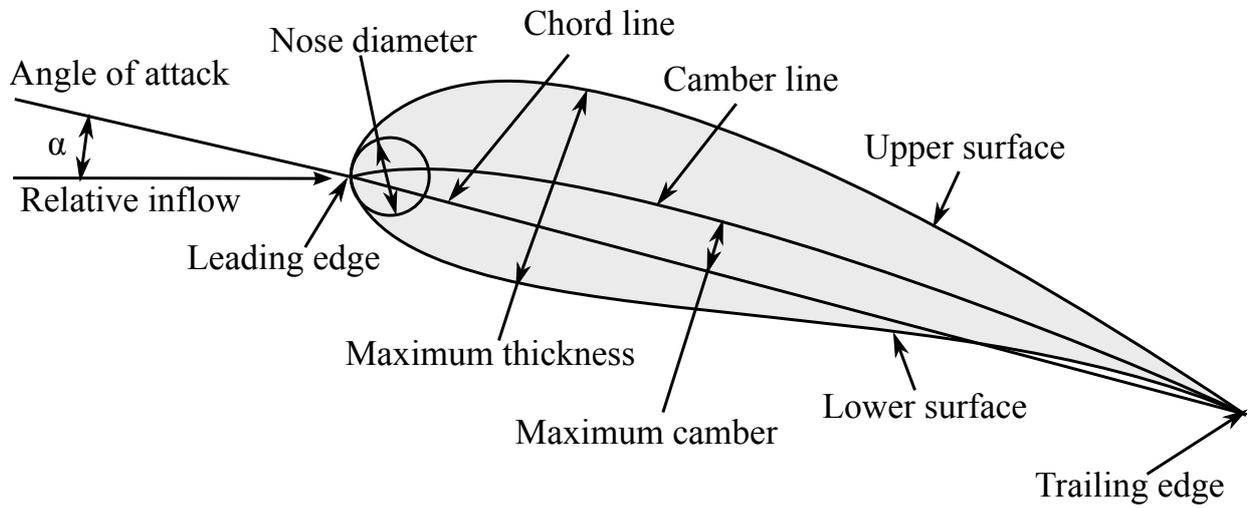
Figure 3: Rudder profile terminology. Adapted from Cleynen (2011)
