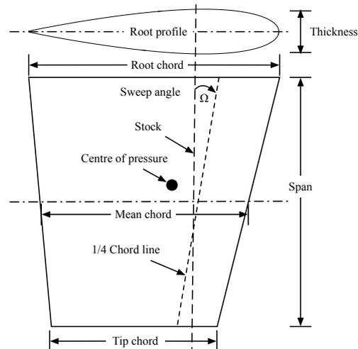
Figure 5: Rudder property terminology. Adapted from Molland and Turnock (2007, p. 72)
