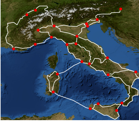
Fig. 5. Interoute network topology with 25 nodes and 35 links.
