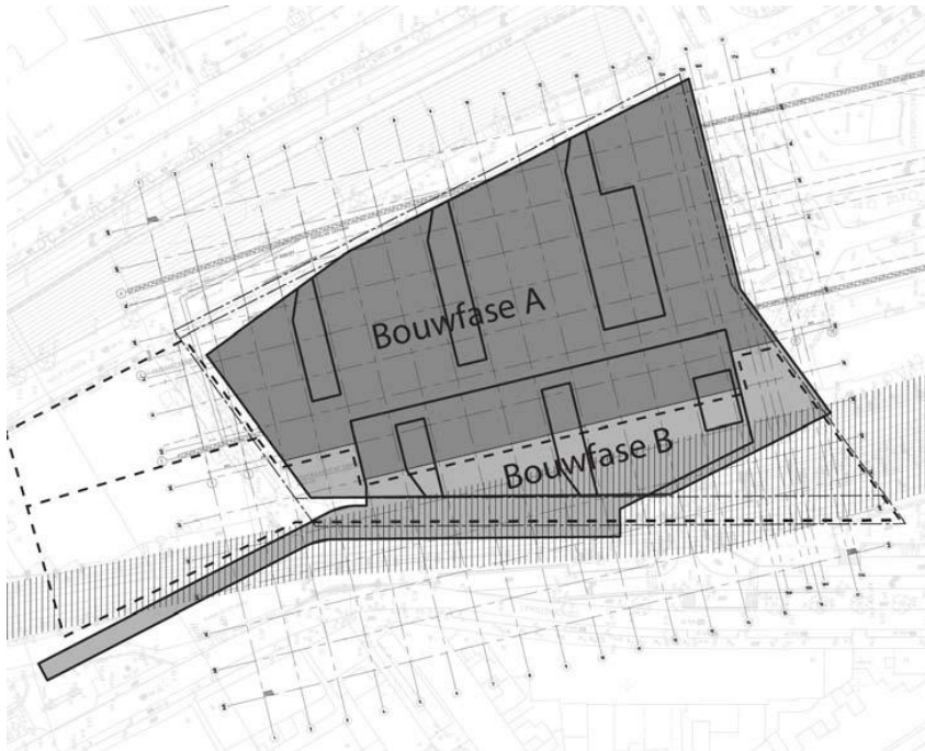
Figure 6-3: Phasing and site accessibility (Mecanoo, 2009)
