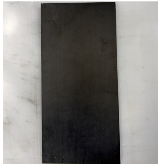
Figure A.9: Trimmed 8 layers laminate
