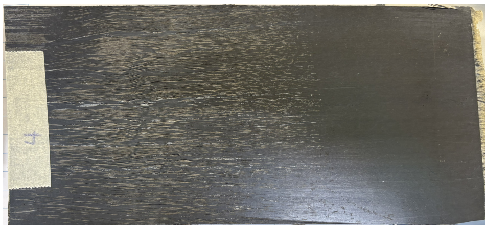
Figure A.6: Defects from hot press process
