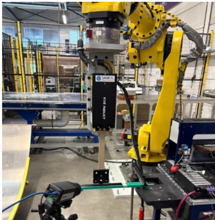
Figure 3.18: Induction welding experiment setup at SAM XL
