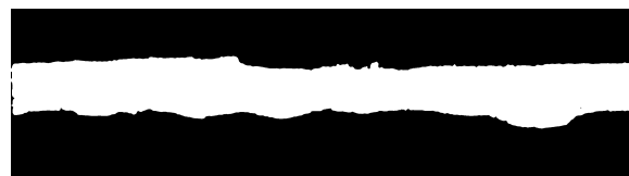
Figure 4.19: Thickness variance mask of DPR tape
