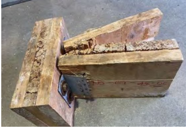
Figure 3.13 Moisture damage and fungal decay in angle bracket connection from Udele research (Udele et al. 2024)
