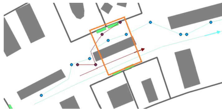
Figure 4-10: Comparison of short and long path: the brown points and vector represent the locations computed by the algorithm and actual path of a short walking, the blue points and vector represent the locations computed by the algorithm and actual path of a long walking.
