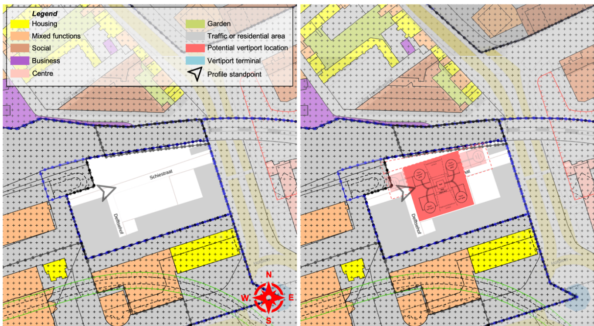
Figure 48 | The location 'Parking 1' and its nearby surroundings as seen from above. The figure shows the existing situation (left) and a possible, new situation with a vertiport fitted in (right). The legend shows the meaning of the different colours. Source: Ruimtelijkeplannen.nl
