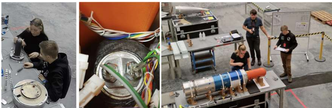
Figure 31: Assembly of the parachute mortar in SPEAR (left), insertion of the gas generator and ignitor bolts (middle), final arming of the SPEAR vehicle through IBF and RBF pins (right)
