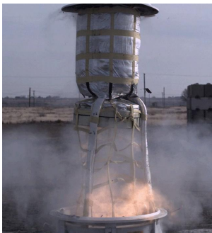
Figure 2.2: Integrated deployment test of the Perseverance parachute mortar [source: NASA]
