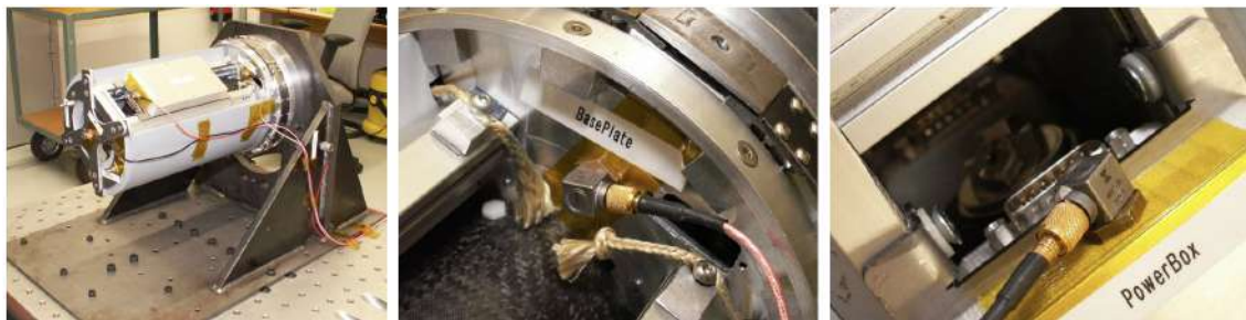
Figure 19: Vibration test 1 [NLR]: SPEAR vehicle (left), parachute mortar in SPEAR (2x right)
