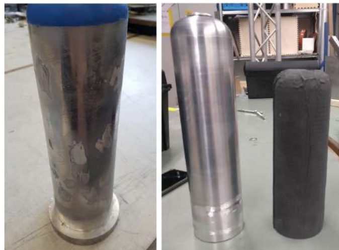
Figure 14: Stratos III mould after putty repair (left) and SPEAR mould (right)
