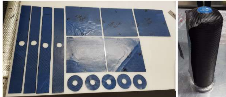
Figure 15: Cut CFRP prepreg shapes (left), canister during layup (right)
