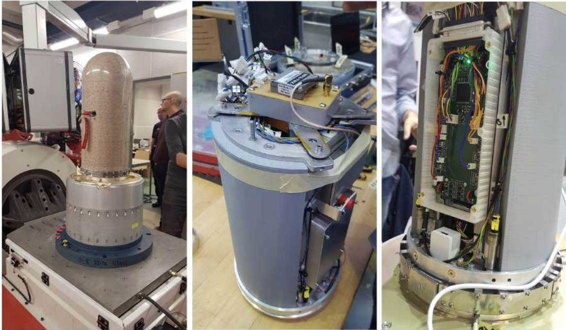
Figure 20: Vibration test 2 [ZARM]: vibration setup (left), inside SPEAR vehicle (2x right)
