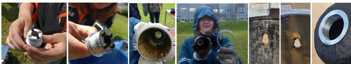
Figure 5.13: Observed failure modes of and damages to the SPEAR mortar
