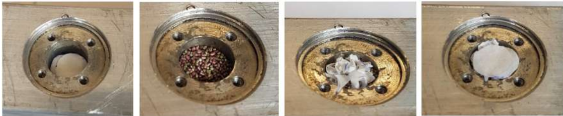
Figure 7: Filling of the gas generator with flash paper and 0.5 grams of NTC
