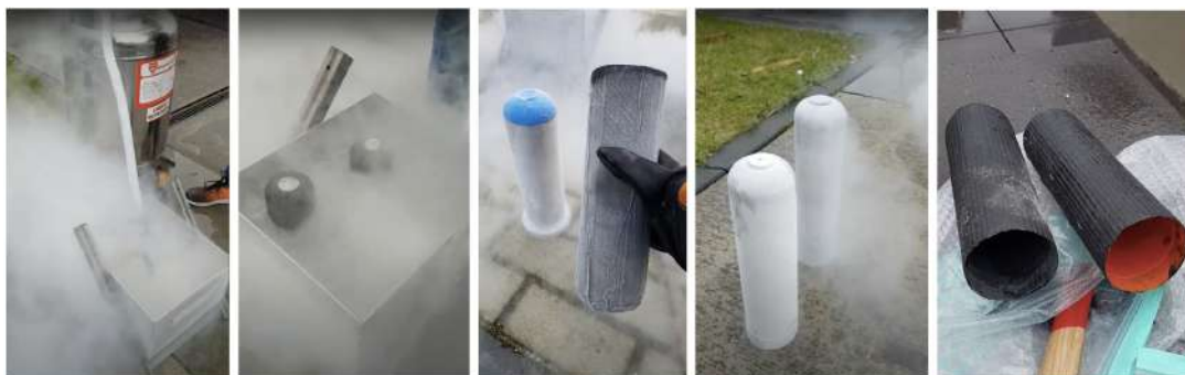
Figure 16: Demoulding of the canisters using Liquid Nitrogen
