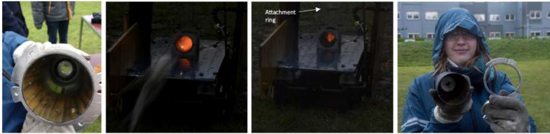
Figure 23: Attachment ring before (left), during (middle x2) and after (right) ejection test 2
