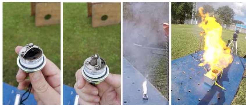
Figure 26: Retainer bolt release (left), ignition of one ignitor bolt and one gas generator (right)
