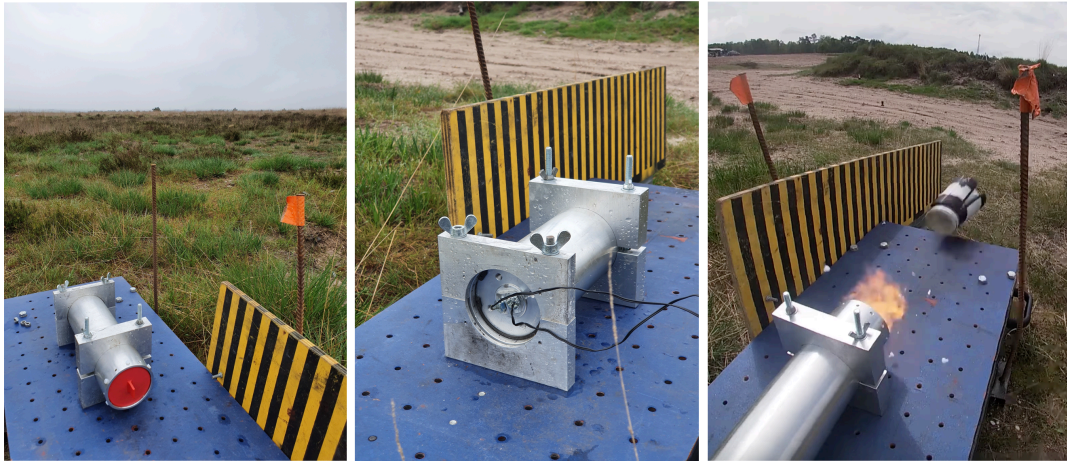
Figure 5.22: Ejection test: test setup front (left), test setup back (middle), parachute ejection (right)
