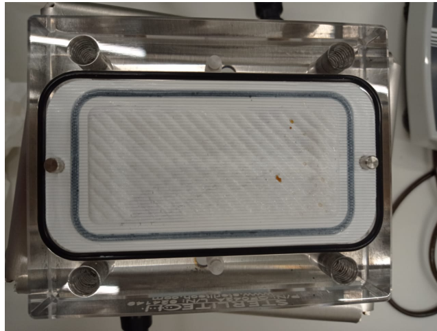
Fig. 4.26: Indication of partial membrane wetting with the appearance of colored droplets on the permeate side of the MD membrane
