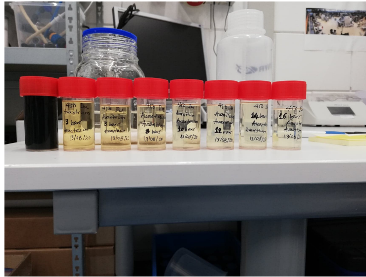
Fig. B.2: Decoloration of the hydrolysate solution with the 450Da ceramic NF membrane for increasing (left to right) pressure values
