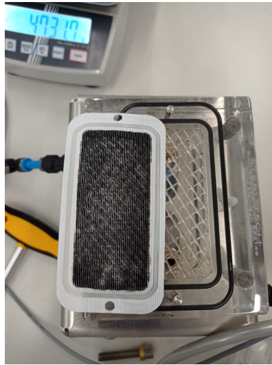
(a) MD membrane after the concentration experiment with the hydrolysate solution
