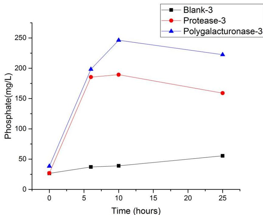
Figure 15: Phosphate release in enzyme batch test 3
