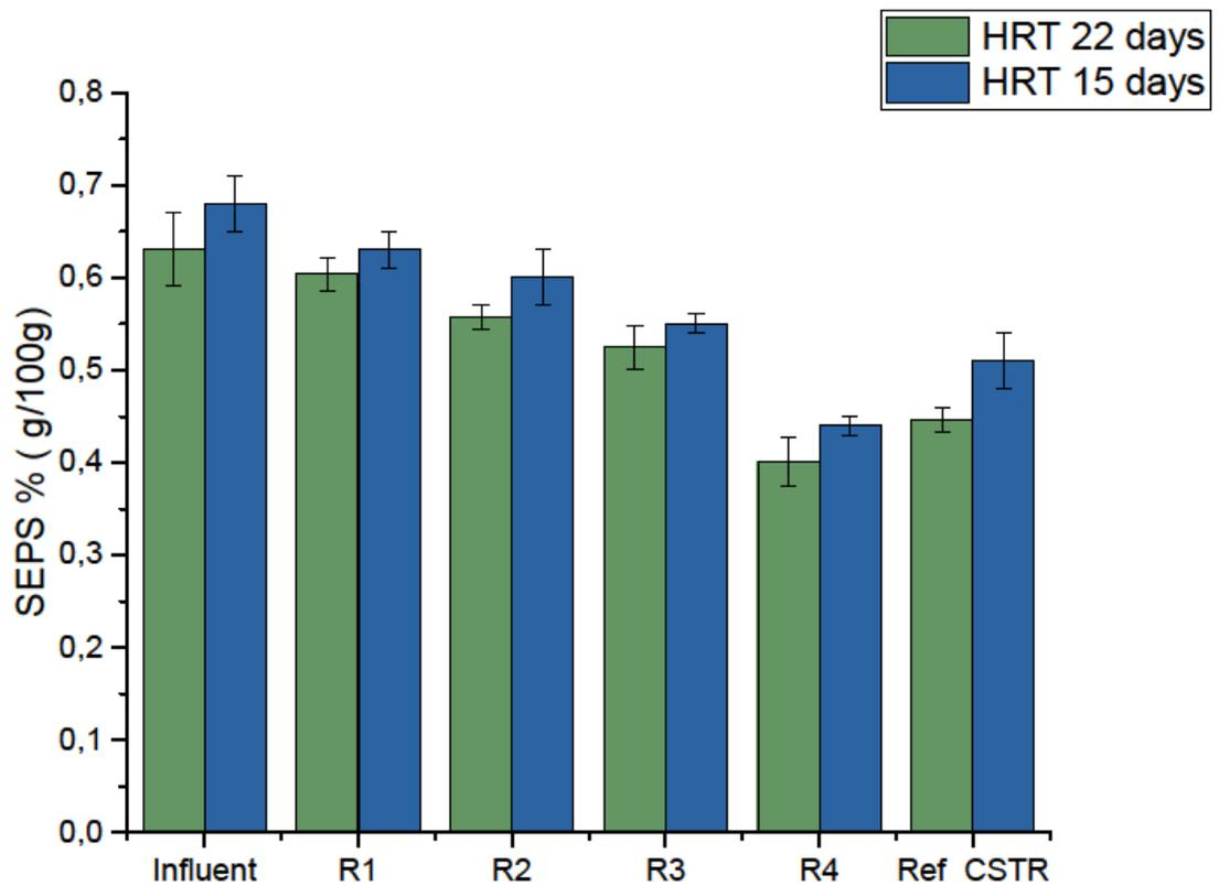
Figure 11: Degradation of structural EPS along Cascade AD and reference CSTR
