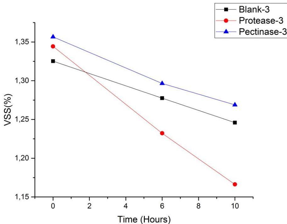
Figure 13: VSS reduction in enzyme batch test-3
