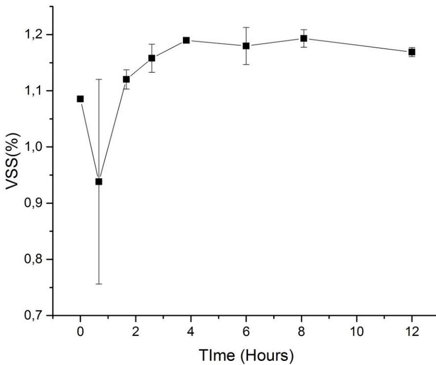
*Appendix figure 8: VSS in Enzyme Batch Test-1 with sludge from secondary sedimentation tank*
