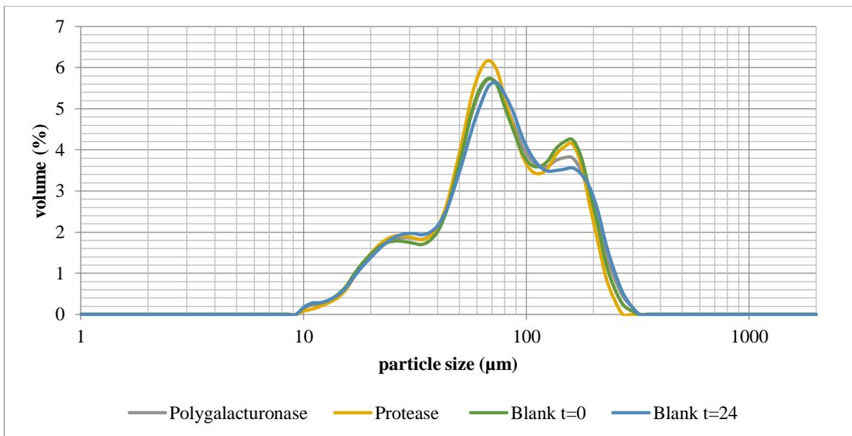
Appendix figure 14: Particle size distribution enzyme batch test 3
