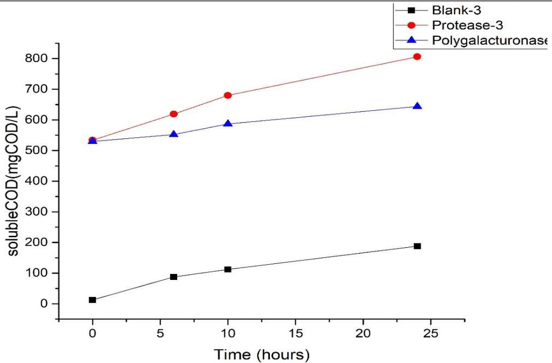
Figure 12: Soluble COD from enzyme batch -3 with B-stage non-bio-P sludge
