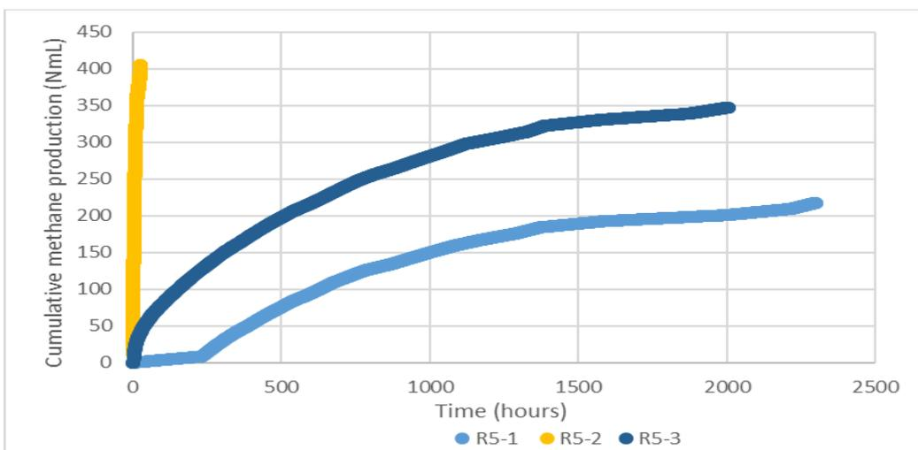
Appendix figure 6 : Methane production from batch test
