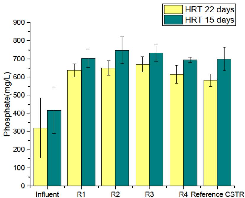
Figure 8: Phosphate release in cascade AD and reference CSTR at HRT 22 and 15 days
