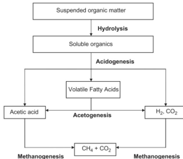
Figure 1: Steps in anaerobic digestion (Appels, Baeyens et al. 2008)
