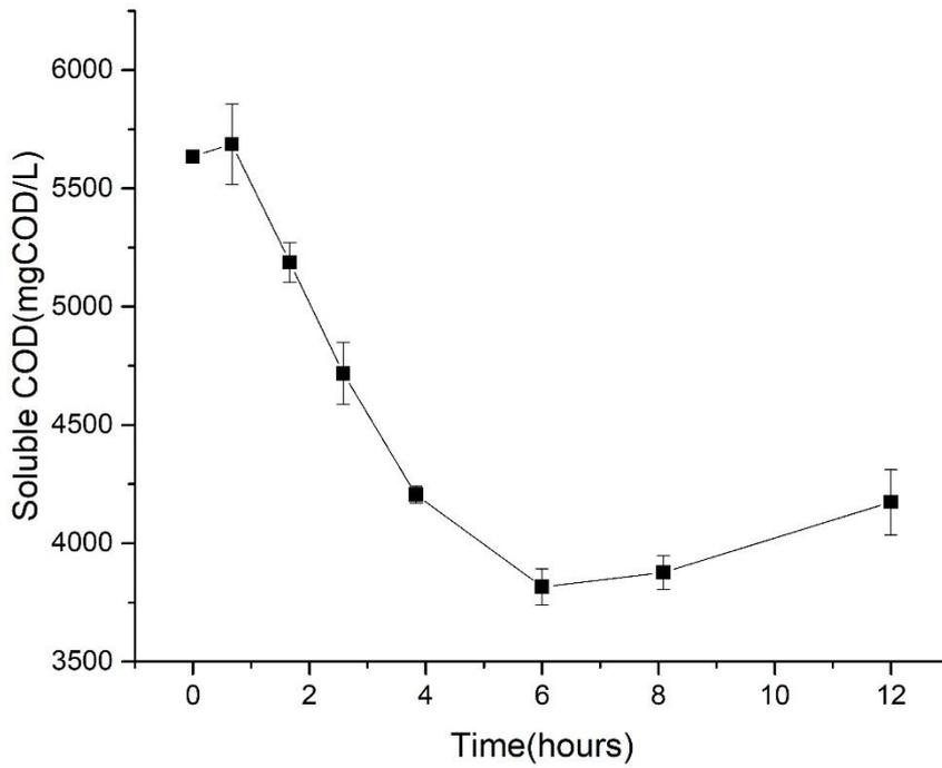
*Appendix figure 7: Soluble COD increase in Enzyme Batch Test-1 with sludge from secondary sedimentation tank*
