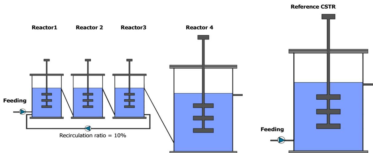
Figure 4: Scheme of the reactor system with cascade AD (left) and reference CSTR (right)
