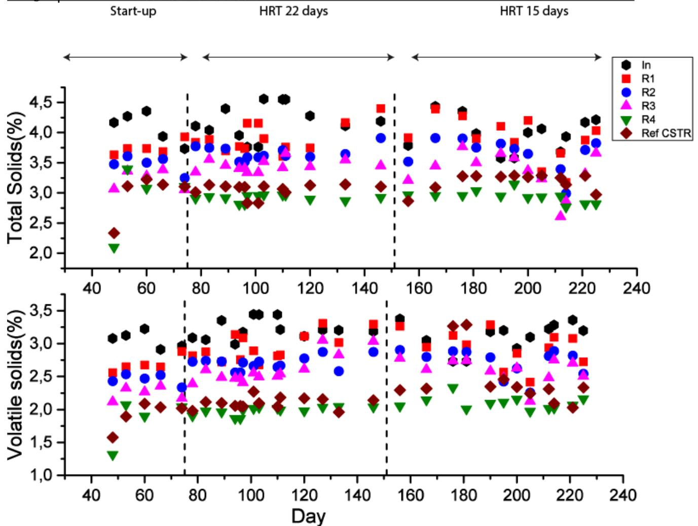
Figure 6: Total and Volatile solids in cascade AD and reference CSTR
