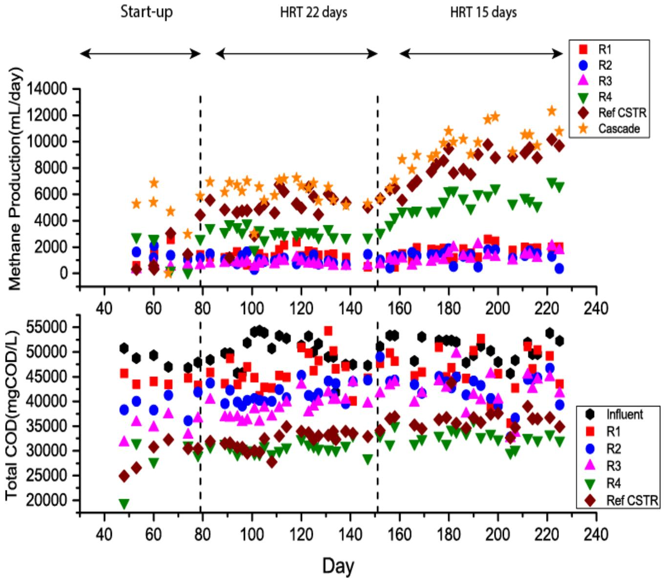
Figure 5: Methane production and TCOD in Cascade AD and Reference CSTR
