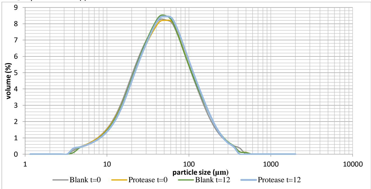
Appendix figure 13: Particle size distribution enzyme batch test 1
