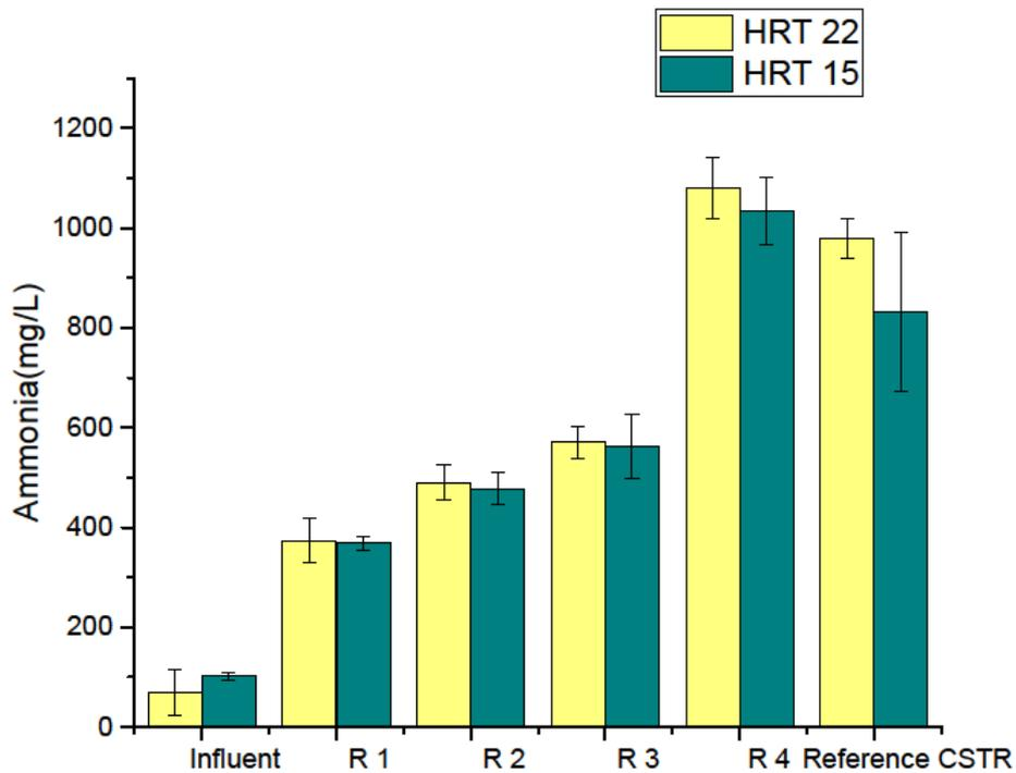
Figure 7: Release of Ammonium in cascade AD and reference CSTR at HRT 22 and 15 days
