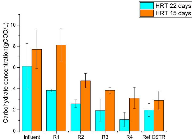
Figure 10: Carbohydrate concentration in cascade AD and reference CSTR
