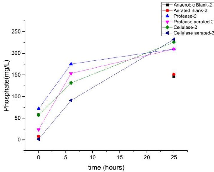
Appendix figure 11: Phosphate release from enzyme batch test-2
