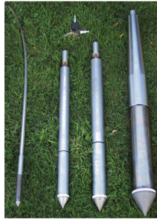
(b) Illustration of various cone penetrometers used for soil data acquisition, taken from [15].
