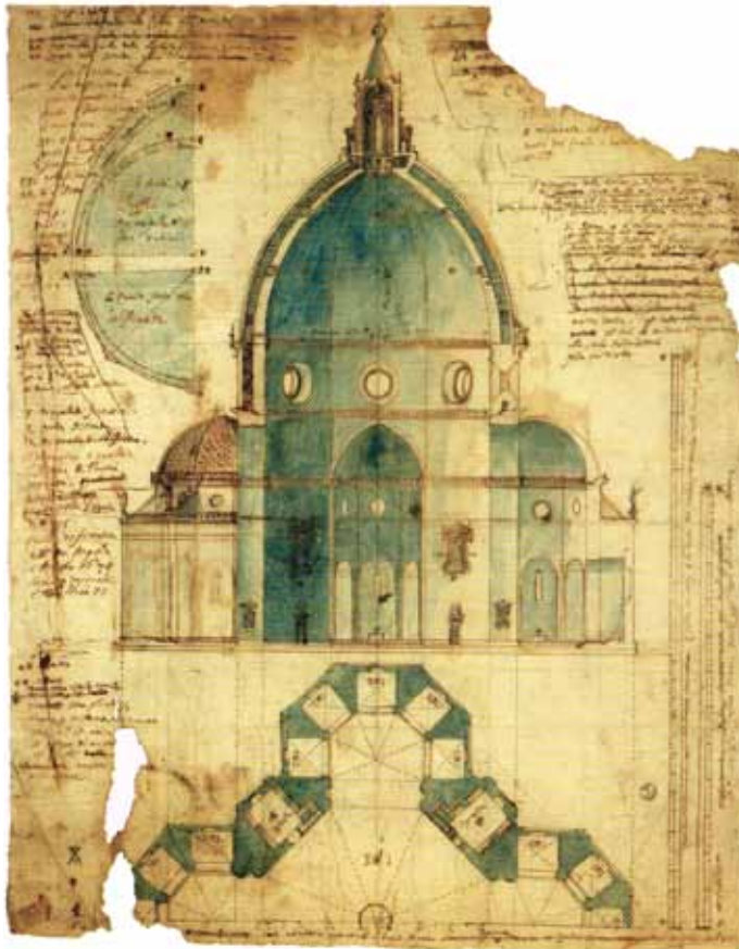
Figure 2.3.2. Cupola del Duomo, late 16th century, as analysed by Lodovico Cardi, also known as il Cigoli, (21 September 1559 - 8 June 1613)
