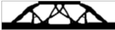
Figure 5.10: Design as optimized with only diagonal sensitivity entries.
