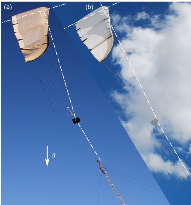
Figure 8. Side view of a kite partially depowered during a landing maneuver (a) and fully powered during a crosswind flight maneuver (b). The photo on the right was taken during a flight test in which the KCU was replaced by a ring that collected the joined power lines and the two steering lines and redirected them as a triplet of parallel lines to the pilot on the ground. The position of this ring is indicated by an overlaid transparent image of the KCU.
