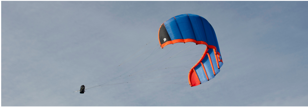
Figure 2. LEI V5.40 kite with 40 \text{ m}^2 wing surface area controlled by a suspended cable robot. This prototype temporarily reached a tether force of 15 \text{ kN} and a mechanical power of 100 \text{ kW} during a test flight in May 2018 (Kitepower B.V., 2018b).
