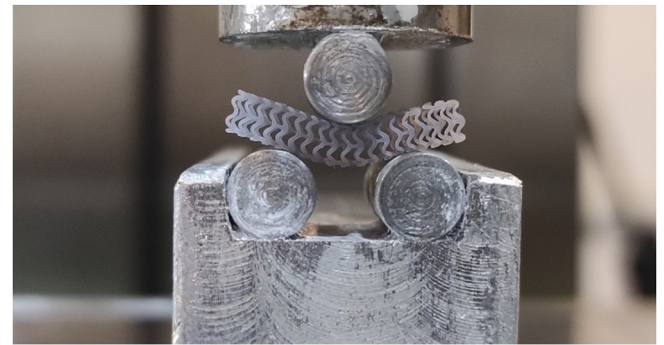
Fig. 9. Experimental test of the three-point bending process.
