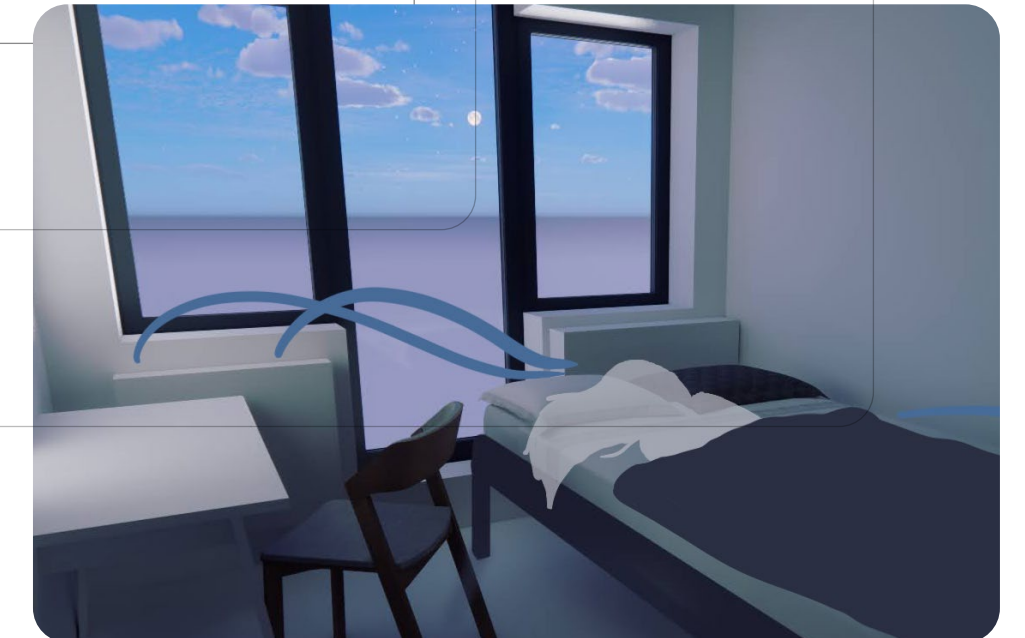
Fig. 7, The cold air from the ventilation goes directly to the sleeping person
