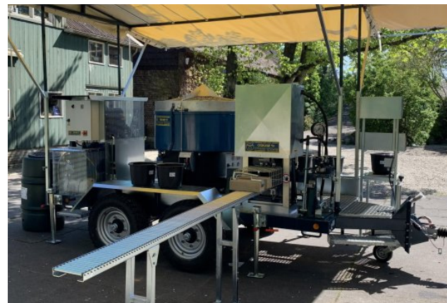
FIGURE 48 On site processing technique for making pressed loam stones
