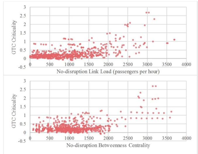
Fig. 3. GTC criticality versus no-disruption link load (top) and betweenness centrality (bottom)
