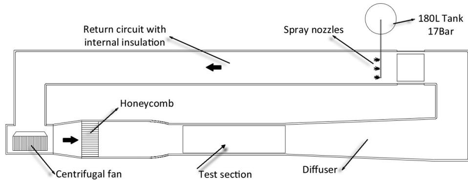
**Figure 9** Schematic view of wind tunnel
