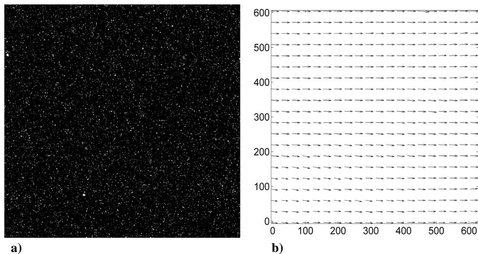
**Figure 10** a) PIV image of fluorescein contained alginate microparticles (600 x 600 pixels; 30 mm x 30 mm) in air by using Nd-YAG green laser with a wavelength of 532 nm b) corresponding velocity vectors.
