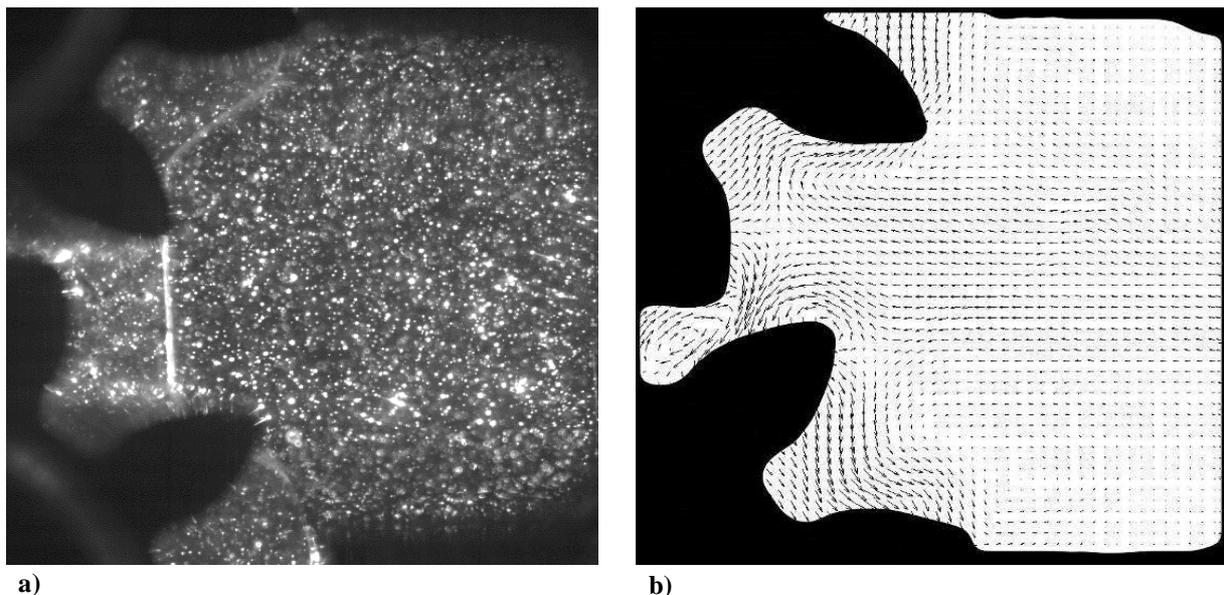
**Figure 8** a) Illumination of alginate microparticles in the suction chamber of an external gear pump. Analyzing fluid is a commercial oil with a density of  $885\text{ kg/m}^3$  and viscosity of  $0.028\text{ Pa}\cdot\text{s}$ , b) Corresponding velocity vectors
