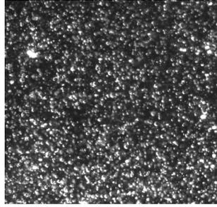
**Figure 5** PIV experiment of the alginate microparticles, engine oil with density of  $885\text{kg/m}^3$  and viscosity of  $0.028\ \mu\text{m}$  has been used as liquid and pulsed infrared diode laser with a wavelength of  $800\ \text{nm}$  has been used as illumination.
