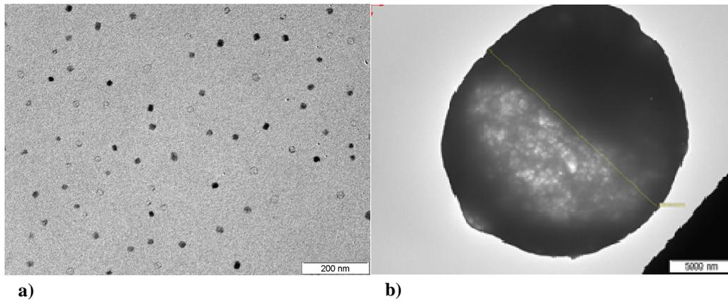
**Figure 1** a) TEM results of dry alginate nanoparticles in 200 nm scale. b) TEM results of wet alginate microparticles in 5000 nm scale
