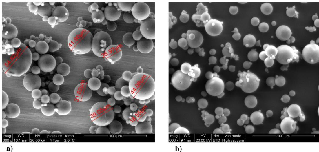
**Figure 3** ESEM images of alginate microparticles in **a)** liquid and **b)** dry form in 100  $\mu\text{m}$  scale.
