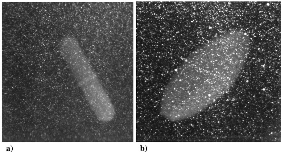
**Figure 6** Illumination of alginate microparticles contains fluorescein by using NdYAG green laser with a wavelength of  $532\ \text{nm}$  **a)** Distilled water has been used as liquid, **b)** Olive oil has been used as liquid
